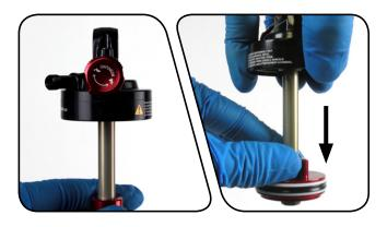
5 Install the seal head/air piston onto the damper body. While holding only the seal head/air piston, thread it completely onto the damper body.
