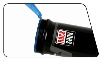
Position the threaded side of the air can over the damper body eyelet. Firmly press the air can onto the seal head/air piston and damper body until the air can is approximately 30 mm from the shaft eyelet threads.
