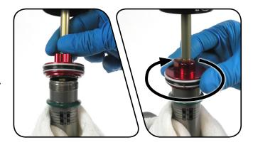
6 Use a torque wrench with 17 mm crowfoot socket to tighten the seal head/air piston to 28 N·m (250 in-lb).
