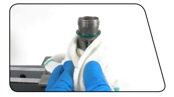
Pour RockShox 3wt suspension fluid into the the damper body until it is level with the top of the damper body. Use your finger to remove any bubbles from the surface of the fluid.
