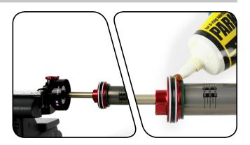
Apply a small amount of blue threadlock to the air can threads. Do not get any threadlock on the o-ring; it will prevent the o-ring from sealing properly.
