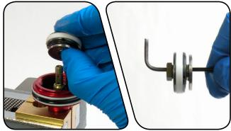
**5** Pull up on the seal head/air piston to remove it from the damper shaft.
