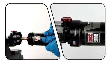
5 Remove the shock from the vise. Turn it over and clamp the damper body eyelet into the vise, so the shock is vertical.
