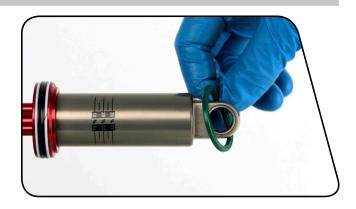
2 Remove the shock from the vise. Turn the shock over and clamp the damper eyelet into the vise, so the shock is vertical.
