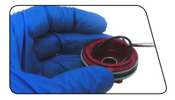
8 Install the seal head/air piston onto the damper shaft with the seal head threads oriented upward.
