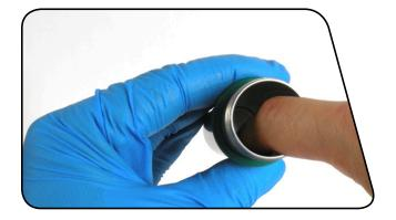
Remove the IFP o-ring. Spray the IFP with isopropyl alcohol and wipe it with a clean rag.
