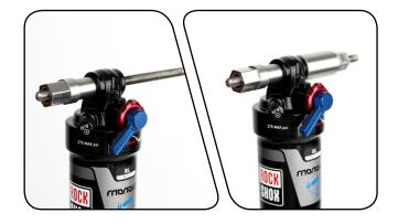
Clamp the catcher in a vise or hold it secure with a 13 mm open end or adjustable wrench.
