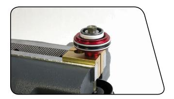
Remove and replace the glide ring located on the main piston.
