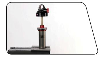
Use a 2 mm hex to unthread and remove the bleed screw, located in the seal head/air piston.
