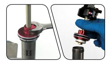
**5** Remove the damper body from the vise and pour the fluid into an oil pan.
