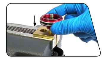
Thread the main piston, by hand, onto the damper shaft. Use a torque wrench with a 10 mm socket to tighten it to 4.5 N•m (40 in-lb).
