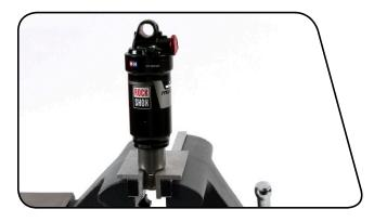
**6** Stabilize the air can with a strap wrench to prevent it from rotating. Use a torque wrench with a 13 mm crowfoot socket to tighten the air can to 17 N·m (150 in-lb).
