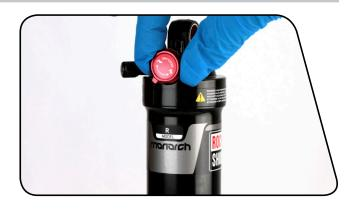
Check and record your current air pressure setting to assist with post-service set up.
