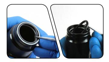
Use your finger or a pick to pull or push the step bushing ring out of the air can.
