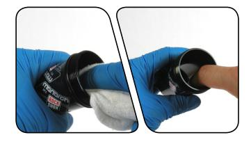
**5** Install the new step bushing ring, quad ring, back-up ring, and dust wiper seal.
