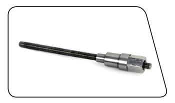
2 Insert the threaded rod through the shaft eyelet until the push pin rests against the bushing pin. Thread the large, open end of the catcher along the rod until it rests on the end spacer.
