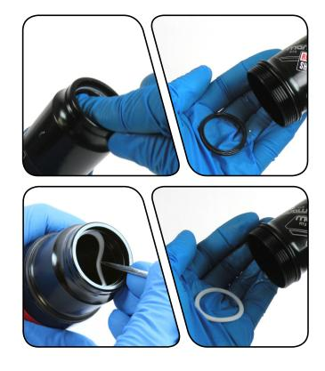
A Spray isopropyl alcohol inside the air can and wipe it with a clean rag. Remove a glove and use your finger to inspect the inside and outside of the air can for scratches, dents, or other surface deformations. Replace the air can if it is scratched or damaged.
