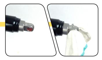
Use a strap wrench to remove the air can. Wrap the strap around the section of the air can furthest from the shaft eyelet. Turn the wrench counter-clockwise to loosen and unthread the air can.
