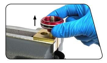
6 Use a pick to remove the seal head/air piston o-ring, located in the interior of the seal head.
