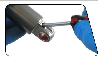
2 Clamp the damper body eyelet into the vise, so the damper body is vertical.
