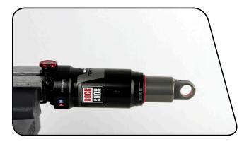
6 If the shock is collapsed so that a minimal amount of damper body is visible, there is still air pressure in the air can. Insert a rag through the damper body eyelet. This will prevent the air can from forcefully ejecting from the shock upon disassembly.
