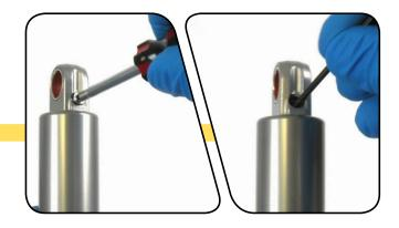
Use a Schrader valve tool to remove the valve core.
