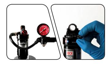
**9** Remove the shock from the vise. Spray isopropyl alcohol on the entire shock and wipe it with a clean rag.
