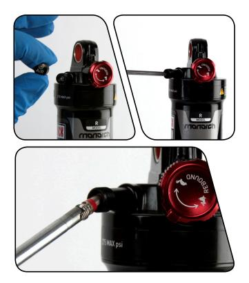
Use a Schrader valve tool to remove the air/nitrogen port cap.
