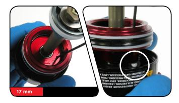
8 Spray the entire shaft and piston assembly with isopropyl alcohol and wipe it with a clean rag.
