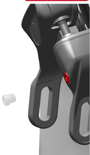
Use a T10 TORX® to tighten the bleed screw to 1.5-1.7 N·m (13-15 in-lb). Clean any DOT fluid that drips from the bleed port with a rag.
