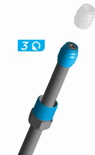
Thread the compression fitting over the hose barb, counter-clockwise, until it is flush or slightly lower than the hose barb.
