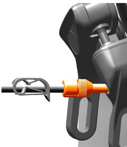
Remove the syringe at the caliper from the bleed port. Clean any DOT fluid that drips from the bleed port with a rag.
