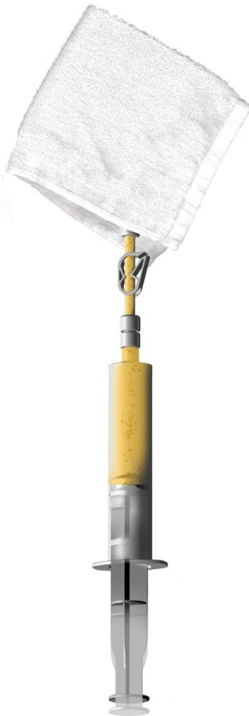
Fill the syringe for the brake caliper with DOT fluid until it is about 1/2 full.
