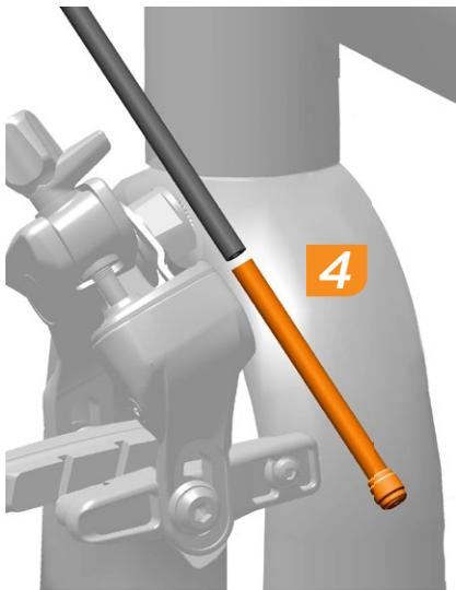
Use a hydraulic hose cutter to cut the excess hose at the brake caliper.
