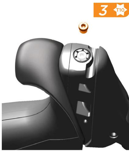
Use a T10 TORX® to remove the bleed screw from the lever. Fluid will come out of the bleed port.
