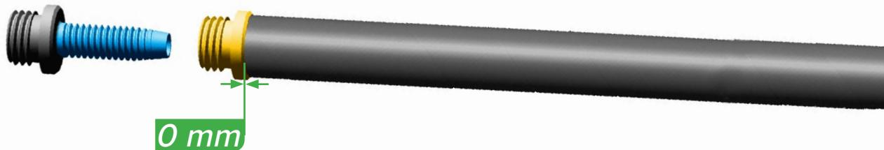
Use a T8 TORX® wrench to thread the SJ hose barb into the hose until it is flush with the end of the hose.
