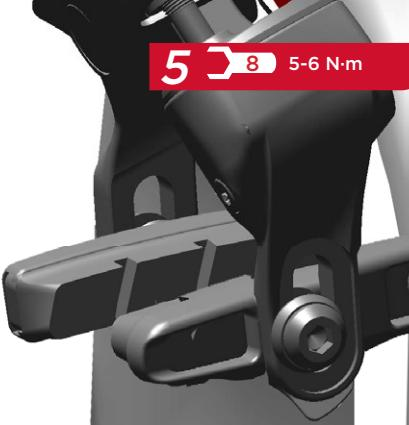
Install the hose firmly into the brake caliper while threading the compression nut by hand. While holding the hose firmly in place, use an 8 mm flare nut wrench to tighten the compression nut to 5-6 N·m (44-52 in-lb).
