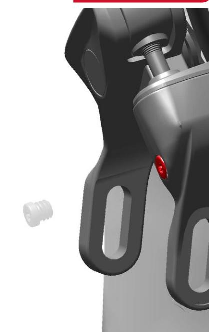
Use a T10 TORX® to tighten the bleed screw to 1.5-1.7 N·m (13-15 in-lb). Clean any DOT fluid that drips from the bleed port with a rag.
