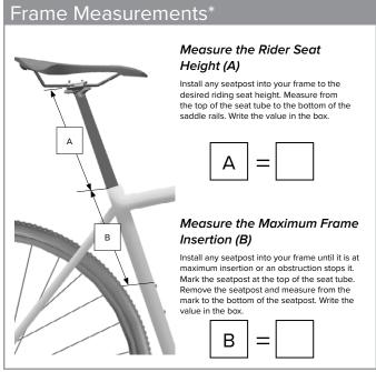
\*Values will vary by rider and frame size. All dimensions are measured in millimeter (mm).
