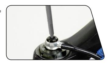
Hold the XLoc button in the extended (locked) position and pull out the syringe plunger. Small bubbles will move into the suspension fluid as air is pulled from the system.
