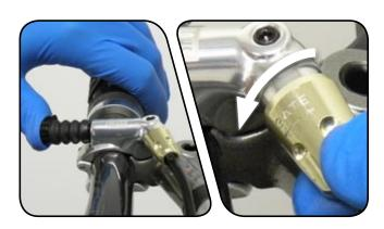
Assemble two RockShox Speed Lube Kit syringes: Install an o-ring onto the end of the brass fitting. Insert the brass fitting into the plastic tube. Insert the red fitting into the other end of the plastic tube. Thread the red fitting into the syringe.
