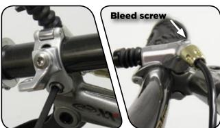
3 Press the XLoc button to set it to the 'Locked' position (button fully extended). Turn the gold Floodgate adjuster in the direction of the the arrow until it stops (maximum Floodgate).
