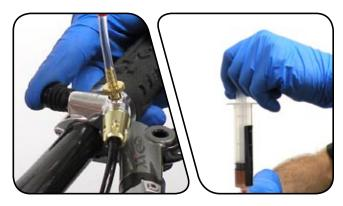
Push in on the syringe plunger, and then press in the XLoc button to release it to the locked position. t
