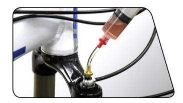
**8** Gently push in the syringe plunger to fill the system with suspension fluid.
