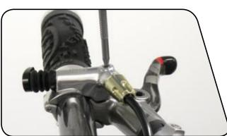
Apply a few drops of suspension fluid to the XLoc bleed port, and then thread the brass fitting of the other speed lube kit into the bleed port.
