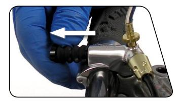
Continue pulling out on the Speed Lube syringe plunger. Push in the XLoc button to the unlocked position. This will dislodge more bubbles from the remote into the syringe.
