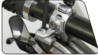
2 Use a T25 TORX wrench to loosen the XLoc handlebar clamp, position the XLoc so that the bleed screw is slightly above the button, and re-tighten the clamp bolt.
