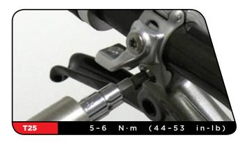
Attach the XLoc shifter to the XLoc bracket with the shifter mounting bolt. Use a T25 TORX wrench to torque the shifter mounting bolt to 2.8-3.4 N·m (25-30 in-lb).
