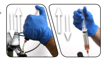
Unthread the syringe from the damper, and use a T10 TORX wrench to re-install the bleed screw into the damper. Use a rag to wipe off any excess suspension fluid.
