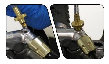
Hold both syringes upright and depress the plunger of the damper syringe while simultaneously pulling out on the plunger of the remote syringe. Reverse this process and repeat until no more bubbles move into the remote syringe.
