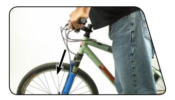
6 Thread a shock pump onto the air valve at the top of the non-driveside fork leg. Pressurize the fork to 20 psi. This is just enough pressure extend the fork to it's full length).
