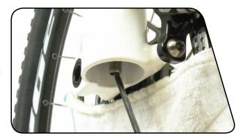
3 Thread a shock pump onto the air valve at the top of the non-drive side fork leg. Use the air pressure chart to determine the appropriate positive pressure for your weight (including riding gear). Use the pump to adjust the positive spring to this pressure.
