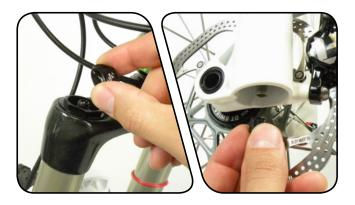
2 While holding a rag over the front brake rotor (if applicable), use a small hex wrench to depress the Schrader valve at the bottom of the fork leg to release all of the air pressure from the negative spring.
