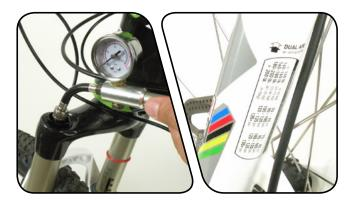
Once you have adjusted the positive spring pressure, remove the pump from the fork, then thread it onto the negative spring air valve, located at the bottom of the fork leg. Inflate the negative spring to the same pressure as the positive spring. Remove the pump from the negative spring air valve.
