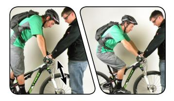
**5** While remaining seated, slide the indicator o-ring or zip tie down against the wiper seal. Avoid compressing the suspension after the o-ring/zip tie is in place.
