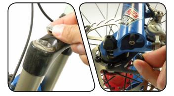
While holding a rag over the front brake rotor (if applicable), use a small hex wrench to depress the Schrader valve at the bottom of the fork leg to release all of the pressure from the negative spring.
