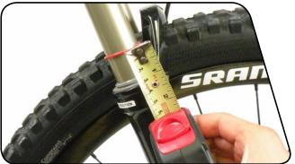
If the fork does not sag the desired amount, you will need to adjust the air pressure settings.
