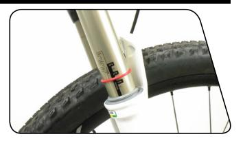
Remove the caps from the air valves located at the top and bottom of the non-drive side fork leg.
