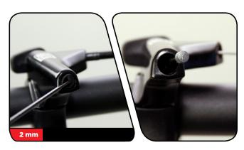
Pull the cable head to remove the cable from the remote system.
