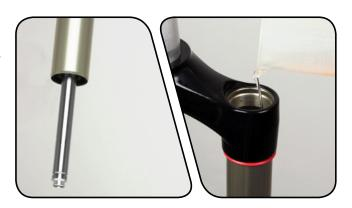
Turn the hex shaft to the unlocked position. Insert the compression damper into the upper tube. Press down and rock side to side until the damper is installed.
