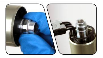
2 Remove the rebound damper and seal head assembly from the upper tube.
