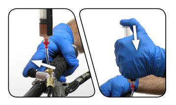
Repeat steps 13-15 until air bubbles no longer move into the hydraulic fluid. It can take several repetitions of this process to fully void the system of air.
