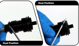
Use a pick to remove and replace the air valve cap o-ring.
