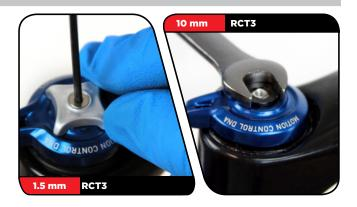
**RLT:** Use a 1.5 mm hex wrench to remove the flood gate set screw. Use your fingers to remove the PTFE seal. Remove the flood gate, compression adjuster knob, and the o-ring on the cam.
