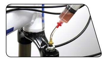
Gently push in the syringe plunger to fill the system with suspension fluid.
