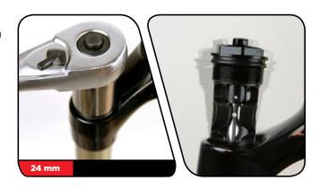
Use a pick or your fingers to remove the compression damper top cap o-ring. Apply grease to the new o-ring and install it.
