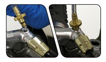
Hold both syringes upright and depress the plunger of the damper syringe while simultaneously pulling out on the plunger of the remote syringe. Reverse this process and repeat until no more bubbles move into the remote syringe.
