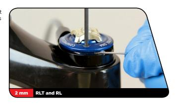
Disconnect the cable from the damper and pull the cable housing off the cable.
