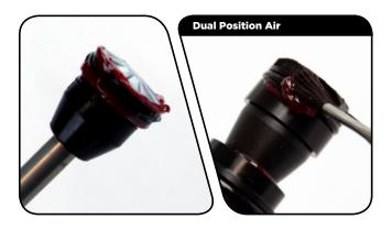
Apply a liberal amount of grease 40-60 mm around the air shaft. Install the floating seal head, a new floating seal head topout bumper, new aluminum support washer, new wavy washer and the air shaft guide, in that order, onto the air shaft.
