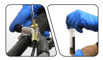
Push in on the syringe plunger, and then push the remote lever until the XLoc button is in the locked (extended) position.
