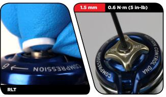
**RL:** Install the compression adjuster knob with the knob dial against the hard stop.
