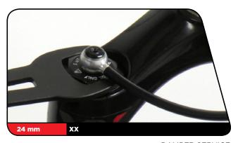
**Remote Only**: Remove the cable from the cable stop collar. Use a 2 mm hex wrench to loosen the cable stop collar clamping bolt. Remove the cable stop collar.
