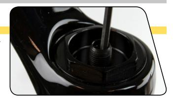
Use a 24 mm socket wrench to remove the air spring top cap. Once removed, clean the upper tube threads with a rag.
