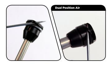
Use your fingers to remove the topout bumper cone from the air shaft.
