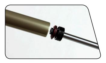
Spray isopropyl alcohol on the inside and outside of the upper tube. Wipe the outside of the upper tube with a rag.
