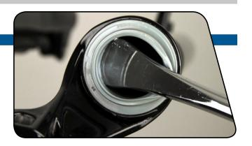
2 Stabilize the lower legs on a bench top or on the floor. Hold the lower legs firmly and use downward force on the tool handle to leverage the dust wiper seal out. Repeat on the other side.
