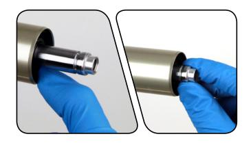
**9** Use internal snap ring pliers to secure the snap ring into the retaining ring groove.
