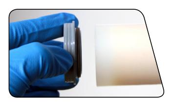
Hold one of the lower legs and use the seal installation tool to push the dust wiper seal evenly into the lower legs until there is no gap between the dust wiper seal and lower legs.
