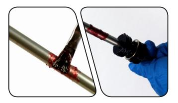
Firmly push the air shaft assembly into the bottom of the upper tube while gently rocking the air shaft side to side.
