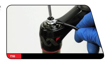
Push the remote lever until the XLoc™ button is in the locked (extended) position and pull out the syringe plunger. Small bubbles will move into the hydraulic fluid as air is pulled from the system.
