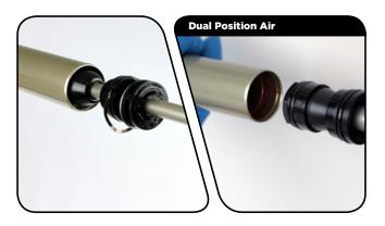
Spray isopropyl alcohol on the inside and outside of the upper tube. Wipe the outside of the upper tube with a rag.
