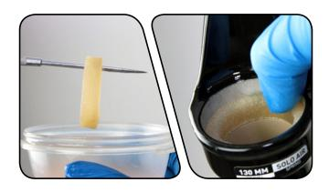
Use a seal installation tool to install the new dust wiper seal. Position the dust wiper seal into the recessed side of the tool, so the grooved side of the seal is visible.
