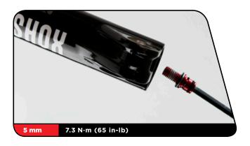
8 Insert the external rebound damper knob into the rebound damper shaft bolt until it is secure. Adjust the rebound.
