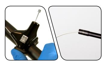
Pull the cable until the cable head is seated in the remote lever.
