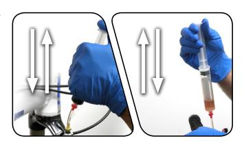
Remove the syringe from the damper, and use a T10 TORX wrench to reinstall the bleed screw into the damper. Use a rag to clean off any excess hydraulic fluid.
