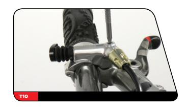
Apply a few drops of hydraulic fluid to the XLoc bleed port, and then thread the brass fitting of the other Speed Lube kit into the bleed port.
