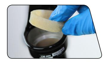
Soak the new foam rings in RockShox 15wt suspension fluid.
