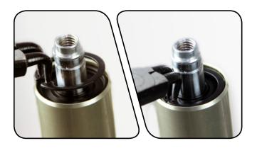
Clamp the fork vertically in the bicycle stand. Pull the rebound damper shaft down to the fully extended position.
