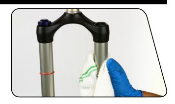
2 Apply a liberal amount of Buzzy's® Slick Honey bike grease to the inner surfaces of the dust wiper seals.
