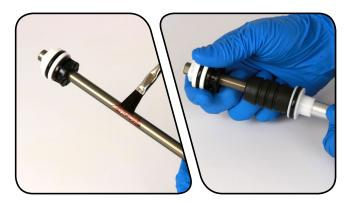
Apply grease to the inside of the upper tube, from the end of the tube (opposite the crown) to approximately 60 mm into the tube.
