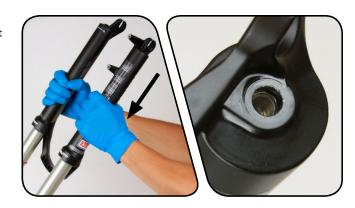
Clean the shaft bolts, crush washers, and crush washer retainers. Inspect the crush washers and retainers. If the crush washers or retainers are flattened or deformed, replace them with new ones.
