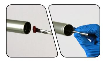
Apply grease to the air piston o-ring and the negative piston outer o-ring.
