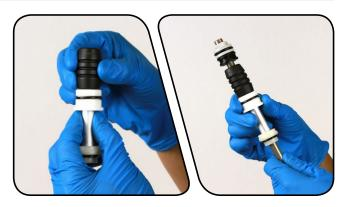
Apply grease to the inside of the air tube, from one end of the tube to approximately 60 mm into the tube.
