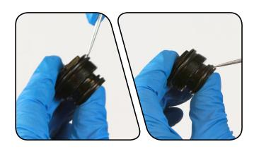
Press the air top cap into the air tube. Apply a small amount of grease to the top cap threads.
