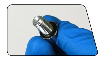
Insert the shaft bolts into the threaded shaft ends through the shaft bolt holes. Use a torque wrench with a 5 mm hex bit socket to tighten the bolts to 7.3 N·m (65 in-lb).
