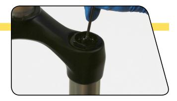
Remove the external rebound adjuster knob by pulling it from the shaft bolt at the bottom of the right fork leg.
