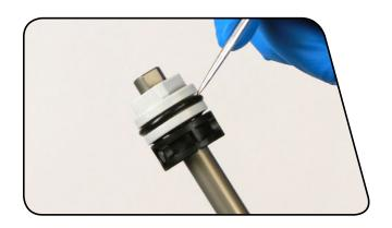
Remove the top out bumper from the negative piston. Use a pick to remove the inner and outer negative piston o-rings. Apply grease to the new o-rings and install them. Install the top out bumper onto the negative piston.
