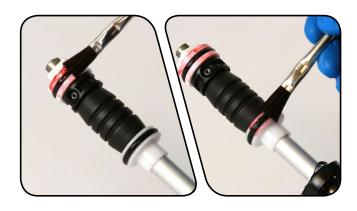
${\bf 11}$  Firmly push the air assembly into the bottom of the upper tube while gently rocking the air shaft side to side.
