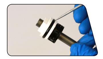
Remove the top out bumper from the negative piston. Use a pick to remove the inner and outer negative piston o-rings.
