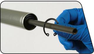
Firmly pull on the air shaft to remove the air spring assembly from the upper tube. Clean and inspect the assembly for damage.
