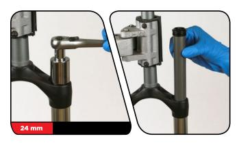
Remove the top cap from the air tube assembly.
