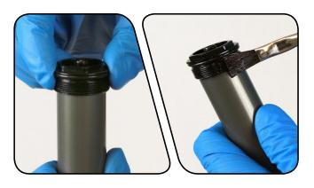
Insert the air assembly, shaft first, into the top of the upper tube. Guide the air shaft through the shaft guide in the bottom of the upper tube. Check the bottom of the upper tube to make sure the air shaft guide is seated into the upper tube shaft guide.
