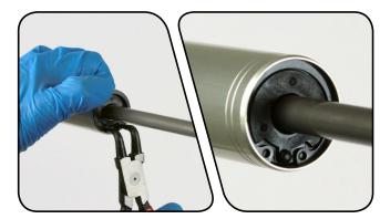
Use a pick to remove the top cap o-ring. Apply a small amount of grease to a new top cap o-ring and install it. Apply a small amount of grease to the top cap threads.
