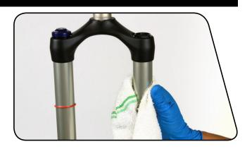
2 Saturate the foam rings with 15 wt RockShox suspension fluid. Apply a small amount of grease to the inner surfaces of the dust wipers.
