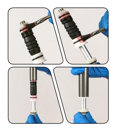
Use a pick to remove the top cap o-rings. Apply a small amount of grease to a new top cap o-rings and install them.
