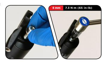
8 Insert the external rebound damper knob into the rebound damper shaft bolt until it is secure. Adjust rebound as desired.
