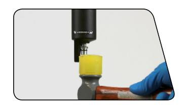
Firmly pull the lower leg downward until oil begins to drain.
