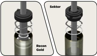
Install the snap ring onto large internal snap ring pliers. Use the pliers to push the base plate into the upper tube while installing the snap ring into its groove. The base plate tab should be situated between the snap ring eyelets.
