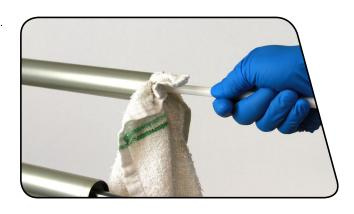
Slide the base plate/negative piston assembly, top out bumper, and travel spacer (if applicable) from the air shaft. Spray the air shaft with isopropyl alcohol and wipe it clean with a rag.
