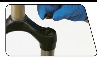
**2** Depress the Schrader valve and release all of the air pressure from the air chamber.
