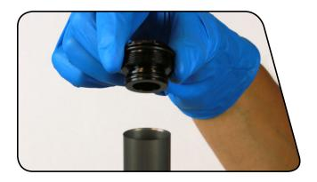
Remove the air shaft/piston assembly from the bottom of the air tube by pulling the shaft down and rocking it from side to side.
