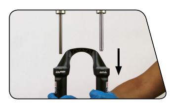
Spray isopropyl alcohol on and into the lower leg. Wipe the lower legs clean, then wrap a clean rag around a dowel and clean the inside of each lower leg.
