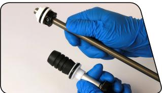
**6** Use a pick to remove the air piston outer o-ring. Apply grease to the new o-ring and install it.
