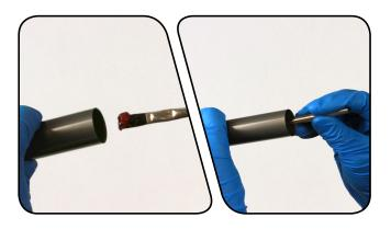
10 Apply grease to the air assembly outer o-rings.
