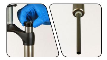
Apply a small amount of grease to the top cap threads and o-ring. Thread the top cap into the upper tube.
