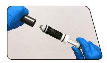
Spray isopropyl alcohol on the inside and outside of the air tube and wipe it with a clean rag. Wrap a clean rag around a long dowel and insert it into the air tube to clean inside the air tube.
