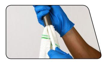
5 Slide the negative piston assembly from the air shaft. Spray the air shaft with isopropyl alcohol and wipe it with a clean rag.
