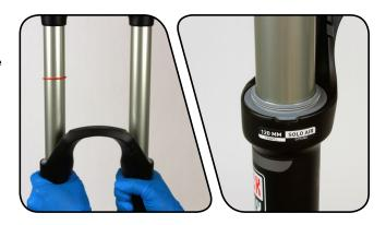
Position the fork at a slight angle with the shaft bolt holes oriented upward, then pour or inject 6 mL of RockShox 15 wt suspension fluid into each lower leg through the shaft bolt hole.
