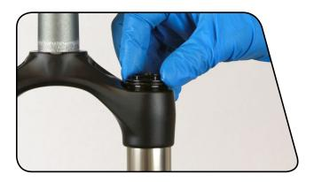
Use a torque wrench and a 24 mm socket to tighten the top cap to  $7.3 \text{ N} \cdot \text{m}$  (65 in-lb).
