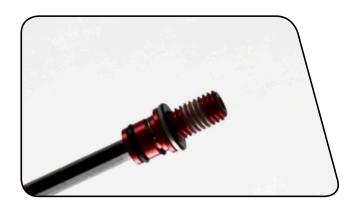
Insert the shaft bolts into the lower legs through the threaded shaft bolt holes.
