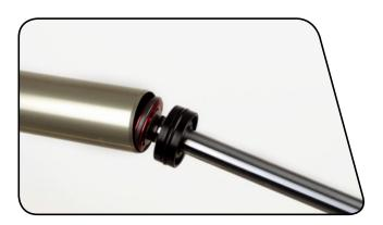
Push the rebound seal head firmly into the upper tube until the retaining ring groove is visible.
