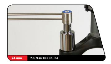
**XLoc™ Remote:** Use a torque wrench with a 24 mm crowfoot to tighten the compression damper to 7.3 N·m (65 in-lb).
