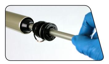
**7** Spray isopropyl alcohol on the inside and outside of the upper tube. Wipe the outside of the upper tube with a rag.
