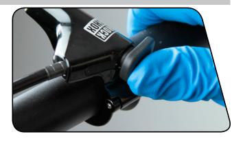
**RLT and RL:** Use a 2 mm hex wrench to loosen the cable pinch bolt on the spool and pull the cable out of the cable end slot. Use pliers to remove the cable end.
