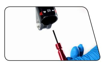
Use a 5 mm hex wrench to loosen both shaft bolts 3 to 4 turns.
