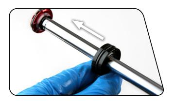
Insert the rebound damper piston into the bottom of the upper tube at an angle with the side opposite the glide ring split entering first. Continue to angle and rotate until the glide ring is in the upper tube.
