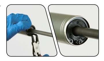
Insert the top cap into the top of the upper tube. Use a torque wrench with a 24 mm socket to tighten the top cap to 7.3 N·m (65 in-lb).
