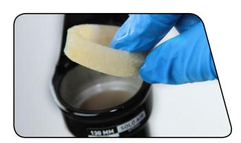
Soak the new foam rings in RockShox 15wt suspension fluid.
