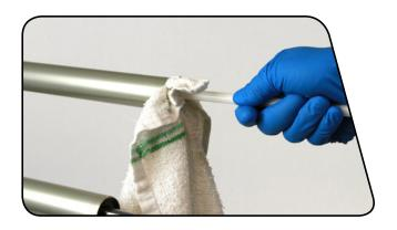
Remove the floating seal head, washers, floating seal head topout bumper, and air shaft guide from the air shaft.
