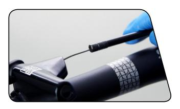
Use a 2 mm hex wrench to open the cable hatch cover.
