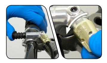
Assemble two RockShox Speed Lube kit syringes:
