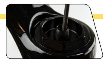
Use a 24 mm socket wrench to remove the air spring top cap. Once removed, clean the upper tube threads with a clean rag.
