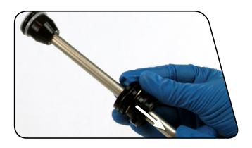
Use a pick to remove the inner and outer floating seal head o-rings.
