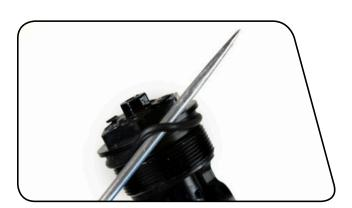
Use a pick or your fingers to remove the compression damper piston o-ring. Apply suspension fluid to the new o-ring and install.
