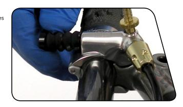
Continue pulling out on the Speed Lube syringe plunger. Push in the remote lever to the unlocked (compressed) position. This will dislodge more bubbles from the remote into the syringe.
