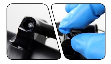
**RLT and RL:** Wrap the cable around the spool and insert it through the cable fixing port. While firmly pulling the cable, use a torque wrench with a 2 mm bit socket to tighten the cable pinch bolt to **RLT and RL:** Wrap the cable around the spool and insert it through 0.9 N·m (8 in-lb).
