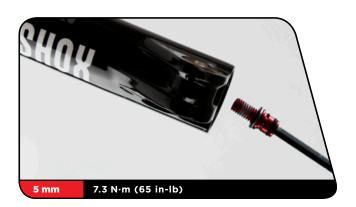
Insert the external rebound damper knob into the rebound damper shaft bolt until it is secure. Adjust the rebound.
