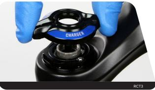
**RC:** Use a 4 mm hex wrench to remove the knob retaining nut. Remove the low speed compression adjuster knob.
