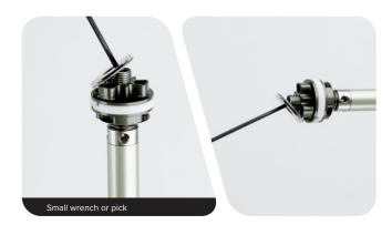
Use the chart below to layout the shim stack for your desired tune on your rebound damper piston. Use a metric caliper to verify the shim outer diameter and shim thickness or print the page at 100% scale to arrange the shim stack using the outlines on the page.
