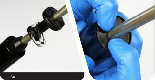
Use your fingers to position the retaining ring into the bottom of the upper tube retaining ring groove. The seal head tab should be positioned between the retaining ring eyelets.
