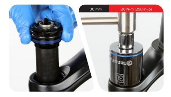
RCT3: Turn the compression cam assembly counter-clockwise until it stops. This is the open position.
