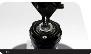
RCT3: Use needle-nose pliers to remove the low speed compression adjuster from the compression top cap.
