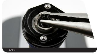
RC: Use needle-nose pliers to remove the bleed plug from the compression adjuster.
