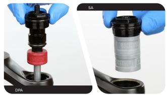
3 Use your fingers or a pick to remove the top cap o-ring. Use your fingers to install a new o-ring. Do not apply grease to the top cap threads.
