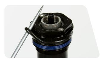
Lightly clamp the cartridge tube into a bicycle stand with the rebound damper shaft oriented upward.
