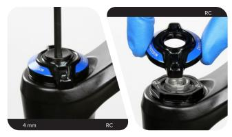
Use a 30 mm socket wrench to loosen the damper top cap. Remove the Charger Damper assembly from the upper tube. Clean the upper tube threads with a rag.
