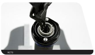
$\ensuremath{\textbf{RC:}}$  Use small retaining ring pliers to remove the retaining ring from the bleed plug.
