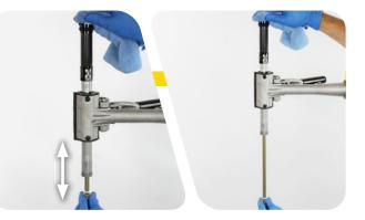
Fill the RockShox Charger bleed syringe half full with 3wt suspension oil and thread the syringe and Charger hose fitting into the compression top cap assembly.
