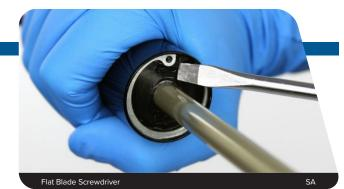
Place your finger over the end of the air spring shaft to prevent it from getting scratched while removing the retaining ring.
