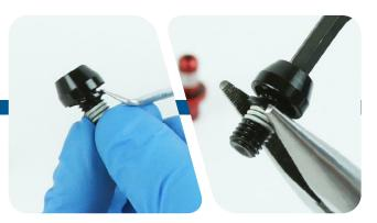
Install a new crush washer on each bottom bolt.
