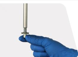
Spray isopropyl alcohol on the damper assembly and clean it with a rag.
