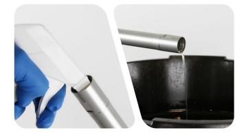
Wrap a rag around a long dowel and insert it into the cartridge tube to clean inside of the tube.
