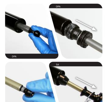
Unthread and remove the bottom bolt from the air shaft. Clean and inspect the assembly for damage.
