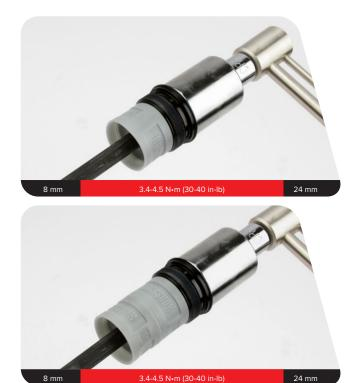
**Dual Position Air:** Install additional Bottomless Tokens onto the DPA air spring shaft, as desired.
