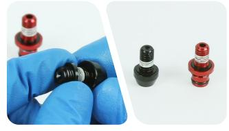
Thread the black bottom bolt into the spring side lower leg. Thread the silver bottom bolt into the damper side lower leg.
