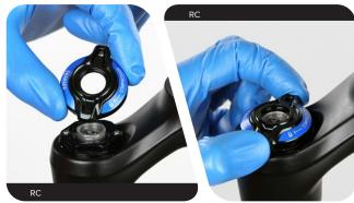
**RC:** Place the low speed compression adjuster knob onto the compression top cap with the long tab near the **back** of the crown. Turn the knob **counter-clockwise** until it engages the first detent space.
