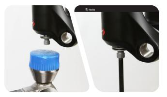
6 Firmly pull the lower leg downward until oil begins to drain. Continue pulling downward to remove the lower leg from the fork.
