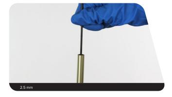
Insert the rebound damper piston into the tube and thread the seal head into the tube by hand.
