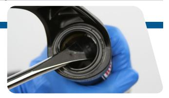
Stabilize the lower leg on a bench top or on the floor. Press down on the tire lever handle to remove the dust wiper seal.
