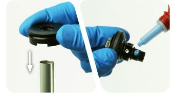
Use your fingers to thread the rebound damper piston onto the rebound damper shaft.
