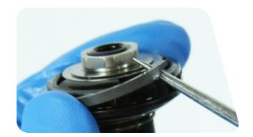
Install the seal head onto the rebound damper shaft with the flat end facing the rebound damper piston.
