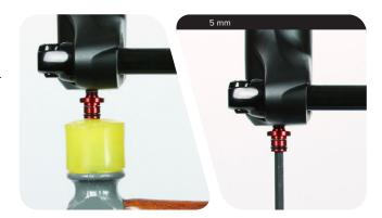
Firmly pull the lower leg downward until oil begins to drain. Continue pulling downward to remove the lower leg from the fork.
