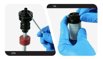
**Dual Position Air:** Push the air shaft into the upper tube to prevent it from getting scratched while removing the retaining ring.
