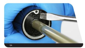
Place your finger over the end of the air spring shaft to prevent it from getting scratched while removing the retaining ring.
