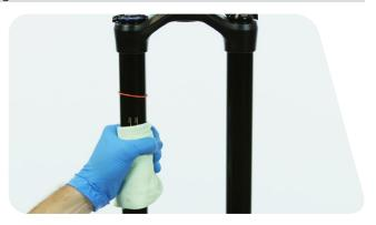
Apply a liberal amount of SRAM Butter grease to the inner surfaces of the dust wiper seals.
