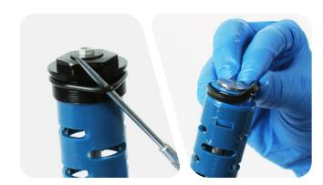
Remove the fork from the bicycle work stand and pour the suspension oil into an oil pan.
