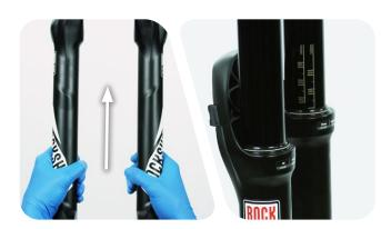
Position the fork at a slight angle with the bottom bolt holes oriented upward. Angle the syringe fitting into each lower leg bolt hole so the oil will only contact the inside of the lower leg and not fill the shaft.
