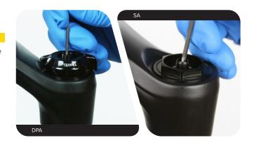
Remove the rebound adjuster knob by pulling it from the bottom bolt.
