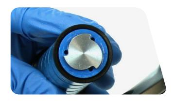
Insert the compression damper into the upper tube. Press down slowly and rock side to side until the damper is installed.
