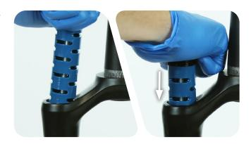
Use a torque wrench with a 24 mm socket to tighten the compression top cap to 28 N•m (250 in-lb).
