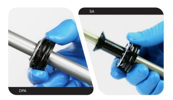
Apply a liberal amount of SRAM Butter grease to the seal head.
