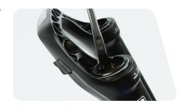
Slide the lower leg assembly onto the upper tube assembly just enough to engage the upper bushing with the upper tubes. The lower leg bottom should not contact the spring or damper shaft.
