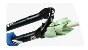
Install the new foam rings into the lower leg.
