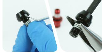
Install a new crush washer on each bottom bolt.
