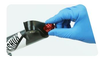
PREFER to the air chart on the fork lower leg and pressurize the air spring to the appropriate pressure for your rider weight.
