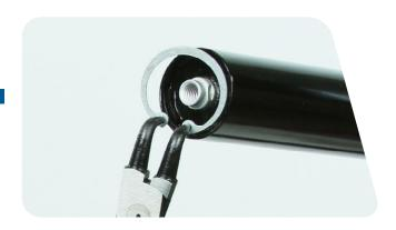
Thread the rebound damper shaft bolt onto the rebound damper shaft 2 to 3 turns. Hold the bolt and pull the rebound damper shaft out of the seal head.
