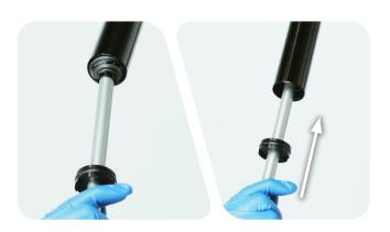
Use your thumbs to push the rebound seal head into the upper tube until the retaining ring groove is visible.
