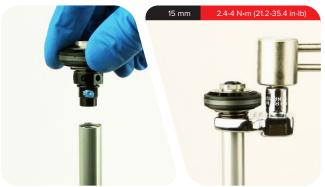
Insert the rebound damper piston into the bottom of the upper tube at an angle with the side opposite the glide ring entering first. Continue to angle and rotate the piston until the glide ring is in the upper tube.
