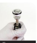
Remove the two o-rings. Clean the shaft.
