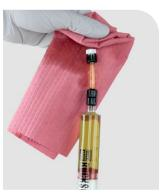
Hold the damper vertically. Thread the syringe into the top cap bleed port.
