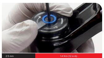
$\ensuremath{\mathsf{RL}}$  R: Install and tighten the cable stop collar with the housing guide oriented forward.
