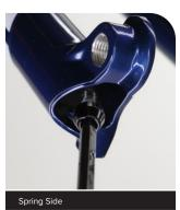
Ultimate / Select +: Use a 10 mm socket and extension to remove the rebound nut on the damper side lower leg.
