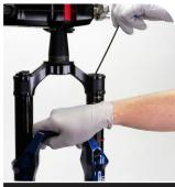
Remove the Schrader valve core from the top cap and set it aside.
