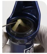
2 Stabilize the lower leg on a bench top or on the floor. Place the tip of a downhill tire lever under the wiper seal. Press down on the downhill tire lever handle to remove the seal.
