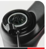
Install the remote spool onto the hex adjuster with the cable set screw oriented  $\approx$ 110 degree from the housing guide.
