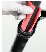
Replace the o-ring or seal with a new one from the service kit. Use your fingers or a pick to pierce and remove the old seal or o-ring.
