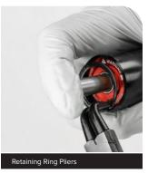
Firmly pull on the air shaft to remove the air spring assembly from the upper tube. Clean and inspect the assembly for damage.
