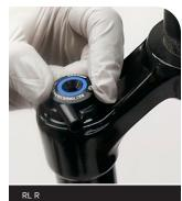
Install and tighten the remote spool retaining screw.
