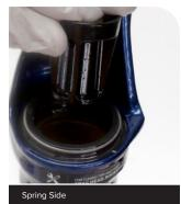
Slide the lower leg onto the upper tube enough to engage the upper bushing with the upper tube.
