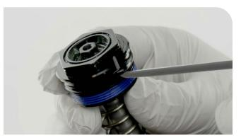
10 Apply grease to the inner seal and bushing in the new rebound damper seal head.
