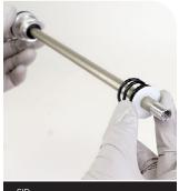
Compress the spring while turning clockwise to thread the spring coil onto the air piston gland. The spring should seat in the air piston.
