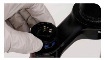
Thread the top cap into the upper tube and tighten it. Press down firmly when tightening the top cap.
