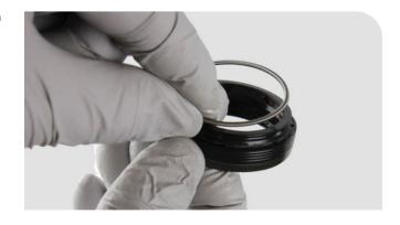
$\mbox{\bf SID SL:}$  Use the 32 mm RockShox Dust Seal Installation tool.
