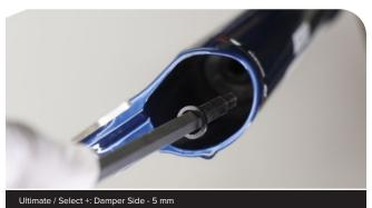
Select/Base: Insert a 5 mm extension or hex wrench into the bolt head of the damper side lower leg. Strike the wrench to dislodge the shaft from the lower leg. The bolt head should contact the bottom of the lower leg. Remove the damper side bottom bolt. Clean the bolt and set it aside.
