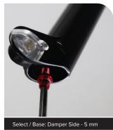
Firmly pull the lower leg downward until fluid begins to drain. Continue pulling downward to remove the lower leg.
