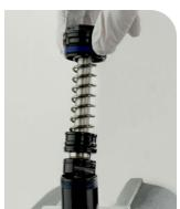
Remove the cartridge tube and rebound damper assembly from the vise and pour the oil into an oil pan.
