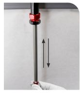
Push the rebound damper into the cartridge tube until the rebound shaft is extended to the 37.5 mm. Do not push the damper into the tube any further.
