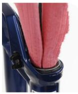
Install the foam rings under the wiper seals.
