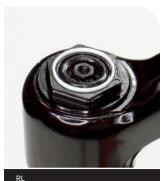
$\mbox{\bf RL}$   $\mbox{\bf R}\mbox{\bf R}$  : Apply grease and install a new glide ring into the groove of the top cap.
