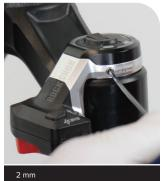
Carefully remove the Flight Attendant Control Module from the compression damper top cap. Use both thumbs to evenly push the Control Module straight up and out of the top cap.
