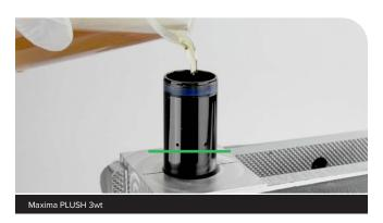
Tie a shop towel around the damper to prevent oil from spilling. Insert the compression damper into the cartridge tube and slowly push it into the tube. The rebound damper will slowly extend as the compression damper is installed; this is normal.
