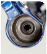
**Ultimate / Select** +: Use a 5 mm wrench to guide the damper shaft through the hole in the lower leg. Push the lower leg further onto the CSU until the damper shaft threads are exposed.
