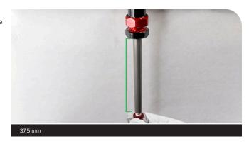
Pour Maxima PLUSH 3wt suspension oil into the tube until the oil is just below the purge holes.
