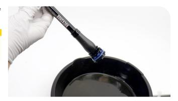
Fill a bleed syringe full with suspension oil. Slowly depress the plunger to remove any air bubbles from the syringe.
