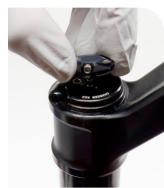
$\mbox{\bf RL}\mbox{\bf R:}$  Loosen the cable stop collar screw and remove the cable stop collar.
