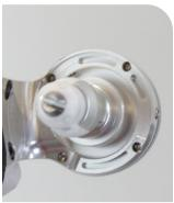
Check key alignment before installation. If the keys are not aligned, rotate the adjuster key on the Control Module output driver to the same orientation as the adjuster key in the compression damper.
