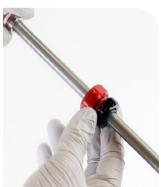
Insert the rebound adjuster knob into the rebound damper and rotate it counter-clockwise until it stops. This is the full open position.
