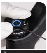
Remove the detent plate. Loosen the adapter knob. Remove the adapter knob.
