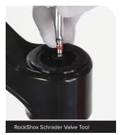
The positive and negative air spring chambers must be FULLY depressurized before removing the air spring top cap assembly.
