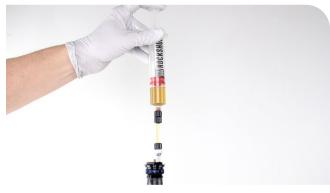
Push the assembly down to compress the rebound shaft. The syringe will fill up.  $\,$
