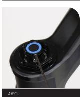
RL R: Loosen the remote spool screw and remove the remote spool.
