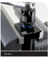
2 Carefully remove the compression damper.
