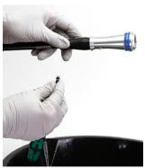
Hold the damper over an oil pan. Compress the rebound shaft to purge the oil from the port in the damper side body. Cycle the rebound shaft to empty the oil from the damper side body.
