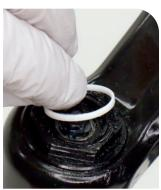
$\mbox{\bf RL}$   $\mbox{\bf R}\mbox{\bf :}$  Loosen the set screw and remove the cable spool and cable stop collar.
