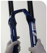
The inside bottom of the lower leg should not contact the spring or damper shafts. A gap between the shaft ends and the lower leg bolt holes should be visible.
