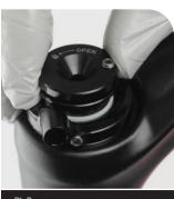
Install and tighten the remote spool retaining screw.
