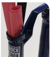
4 Soak the new foam rings in suspension oil. Install the new foam rings into the lower leg.
