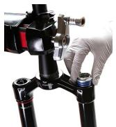
Thread the top cap into the upper tube and tighten it. Press down firmly when tightening the top cap.
