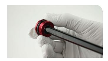
Spray RockShox Suspension Cleaner or isopropyl alcohol into the cartridge tube and clean the inside of the tube with a shop towel and a thin dowel ( $\leq$ 16 mm diameter).
