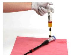
Compress the rebound shaft. The syringe will fill up.
