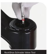
The positive and negative air spring chambers **must be FULLY depressurized** before removing the air spring top cap assembly.
