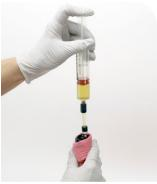
Release the plunger and air will purge into the syringe. Compress and release the plunger to inject oil into the damper. Refill the syringe when necessary.
