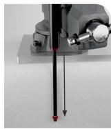
Pour Maxima PLUSH 3wt suspension oil into the tube until it is almost half full. Slowly cycle the rebound damper shaft in and out half way to remove air bubbles trapped under the rebound damper piston. Stop when no bubbles are visible in the oil.
