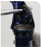
Remove the bottom cup from the lower leg. Remove the jounce bumper from the lower leg, if necessary. Clean the inside and outside of the lower leg.
