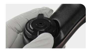
**RL:** Remove the retaining screw and remove the knob. Remove the glide ring and o-ring. Clean the top cap grooves.
