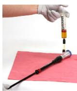
Push the syringe handle down, then release the plunger. Allow the bladder to come to a natural resting position by waiting a few moments until the syringe stops filling.
