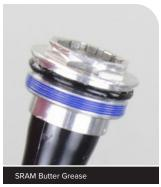
Apply grease to a new inner top cap o-ring and install it.
