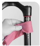
Apply grease to the inner surfaces of the wiper seals.
