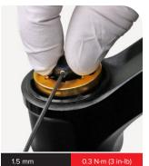
Install the adjuster knob on the top cap so the flange is pointed away from the steerer tube. Rotate the adjuster knob clockwise until it stops on the last detent and the set screw is facing forward. Hold the knob down and tighten the set screw.
