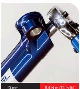
Select / Base: Install the red bottom bolt into the damper side shaft.
