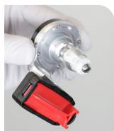
Clean the underside of the Control Module with a damp clean shop towel.
