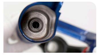
Position the fork at an angle with the lower leg bolt holes oriented upward.
