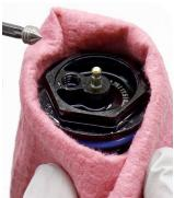
Hold the damper over an oil pan. Compress the rebound shaft to purge the oil from the port in the damper top cap. Cycle the rebound shaft to empty the oil from the damper top cap.
