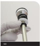
Apply a liberal amount of grease around the air shaft.
