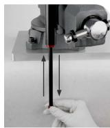
Push the rebound damper into the cartridge tube until the rebound shaft is at the "A" measurement. Do not push the rebound damper into the tube any further.
