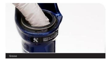
Install the jounce bottom out bumper on the air spring shaft, if necessary. Install the bottom cup, tapered side down, into the spring side of the lower leg.
