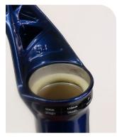
Remove the outer wire spring from each new wiper seal and set them aside.
