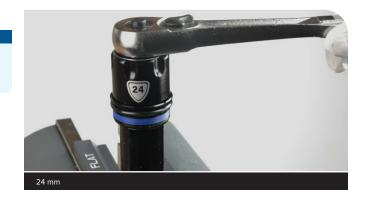
3 Carefully remove the compression damper.
