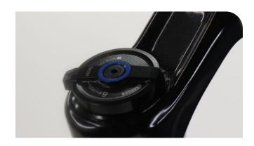
**RL:** Remove the retaining screw and remove the knob.
