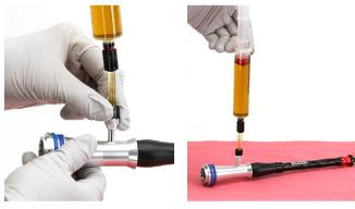
Release the plunger and air will purge into the syringe. Compress and release the plunger to inject oil into the damper. Refill the syringe when necessary.
