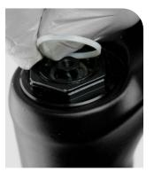
4 Unthread the damper top cap and remove the damper assembly.
