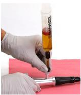
Compress the rebound shaft. The syringe will fill up.
