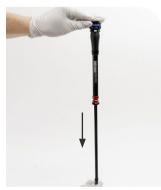
Compress the damper in a vertical position for five minutes. This will allow the remaining bubbles to float to the top.
