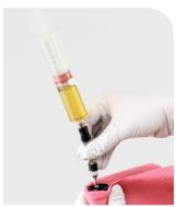
Push the assembly down to compress the rebound shaft. The syringe will fill up.
