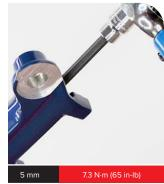
**Ultimate / Select +:** Install the crush washer into the rebound adjuster nut. Install and tighten the rebound adjuster nut onto the **damper side** shaft.
