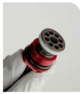
Insert the rebound adjuster knob into the rebound damper and rotate it counter-clockwise 16 clicks from the closed position. This is the full open position.
