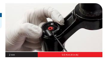
Install the remote spool onto the hex adjuster with the cable set screw oriented within the 20 degree range in the diagram.
