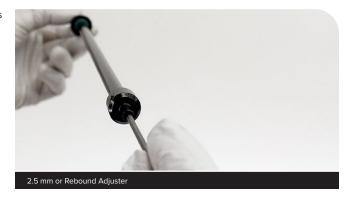
Remove the bleed screw from the top cap.
