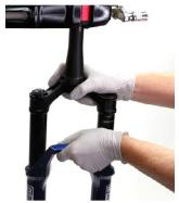
Place an oil pan beneath the fork to catch the draining oil.
