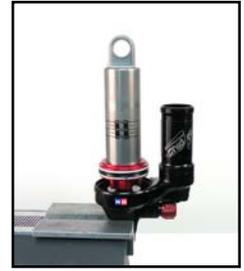
64. Pour additional suspension fluid into the reservoir until it is level with the top of the reservoir.
