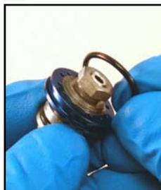
46. Use your fingers to remove and replace the reservoir/shock body o-ring, located at the base of the threads inside the shock body.
