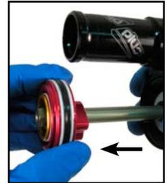
*Do not hold on to the air can eyelet while inserting. It will move the piston/shaft assembly, causing too much fluid to displace out of the damper body.*
