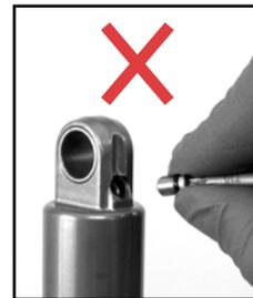
**Do not remove the damper body bleed screw from the damper body eyelet until instructed to do so. Removing the damper body bleed screw while the shock is pressurized will result in fluid being forcefully ejected from the bleed port.**
