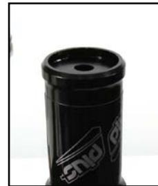
*Keep the reservoir cap square with the reservoir as you install it so that it doesn't bind.*
