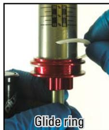
21. Apply a small amount of grease to the air can inner o-ring. Install the o-ring into the small end of the air can, so that it rests on the air can glide ring.
