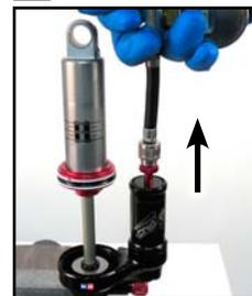
*Once the top cap is resting against the retaining ring, firmly pull up on the adapter to ensure that the retaining ring is completely seated in the groove.*
