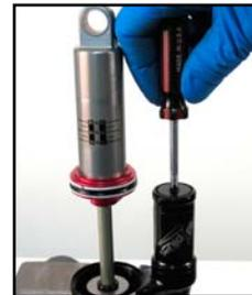
*Once you have pressurized the shock, remove the Monarch air fill adapter from the air fill port BEFORE removing it from the shock pump. Separating the pump from the adapter first will allow all of the air to escape from the shock.*
