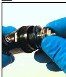
54. Thread the reservoir into the shock by hand. Use a torque wrench with a 27 mm crowfoot socket to tighten the reservoir to 8.4 N-m (75 in-lb).
