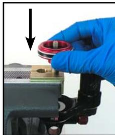
35. Thread the piston assembly by hand back onto the shaft assembly and use a torque wrench with a 10 mm socket to torque it to 4.5 N·m (40 in-lb).
