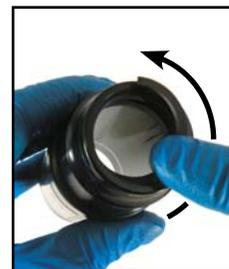
23. Orient the air can dust wiper so that the flat side faces toward the air can and the angled side faces away from the air can. Install the new dust wiper by gently squeezing it into the outer gland at the small end of the air can.
