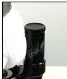
71. Pour additional suspension fluid into the reservoir until it is level with the top of the reservoir.
