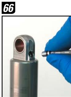
67. Use a pick to remove and replace the damper body bleed screw o-ring. Set the bleed screw aside.
