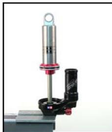
76. Use the Schrader valve tool to install a new Schrader valve into the reservoir top cap.
