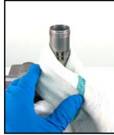
59. Slide the seal head/air piston against the damper piston assembly.
