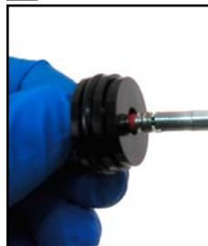
77. Apply a small amount of grease to the reservoir cap o-ring. Push the reservoir cap into the reservoir with the flat side of the cap facing outward, until the cap is just beyond the retaining ring groove.
