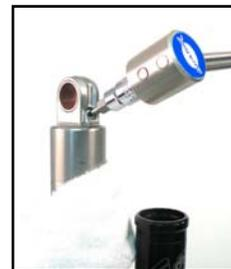
*It may be necessary to fill and purge the damper additional times to completely remove air from the damper body. If this is the case, fill the reservoir with suspension fluid, pull up on the damper body until it stops, then slowly push down on the damper body. Repeat this process until bubbles cease to come out of the bleed port.*
