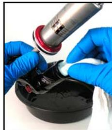
74. Remove the shock from the vise. Pour the remaining fluid out of the reservoir, then wipe the residual out of the reservoir with a clean lint free rag.
