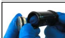
51. Apply a small amount of grease to the IFP o-ring. Press the IFP, with the flat side facing out, into the non-threaded side of the reservoir. Push the IFP into the reservoir to a depth of 35 mm.
