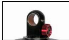
6. Continue to press the bushing until it is completely seated in the eyelet.
