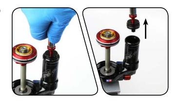
**5** Use your fingers to remove and replace the reservoir cap o-ring.
