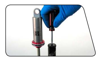
Spray the damper assembly with isopropyl alcohol and wipe it with a clean rag.
