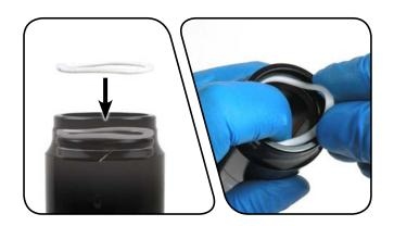
Orient the new dust wiper seal step side up. Install it into the dust wiper seal gland at the top of the air can.
