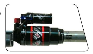
If the shock is collapsed so that a minimal amount of damper body is visible, there is still air pressure in the air can. Insert a rag through the damper body eyelet. This will prevent the air can from forcefully ejecting from the shock upon disassembly.
