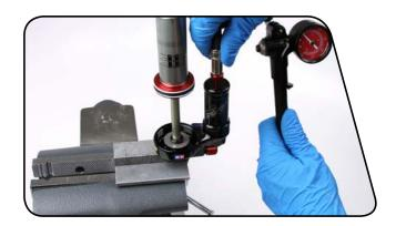
Use the shock pump to pressurize the damper body to 17.2 bar (250 psi).
