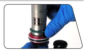
2 Spray the air can threads with isopropyl alcohol and wipe it with a clean rag.
