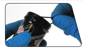
2 Use a pick to pierce the air can dust wiper and o-ring located inside the dust wiper seal gland. Push or pull to remove them, paying attention to the orientation of these parts for reinstallation.
