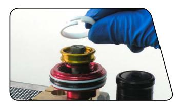
Use a 10 mm wrench to unthread the piston nut. Remove the main piston assembly.
