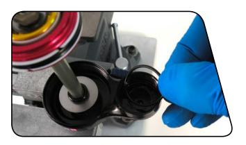
Use your fingers to push the IFP (Internal Floating Piston) out of the non-threaded side of the reservoir.
