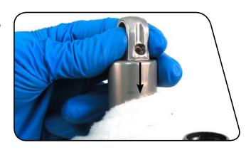
Use a T10 TORX® to install the damper body bleed screw into the damper body eyelet. Use a torque wrench with a T10 TORX socket to tighten the bleed screw to 1.1 N·m (10 in-lb). Wipe the excess fluid from the damper body with a clean rag.
