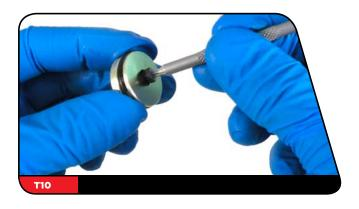
Use a pick to remove and replace the o-ring on the IFP bleed screw.
