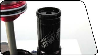
Place one end of the reservoir cap retaining ring into the retaining ring groove in the reservoir, then push around on the ring until it is seated in the groove.
