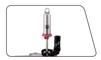
8 Slowly push the damper body downward. Fluid will begin to fill the reservoir through the IFP bleed port. Continue to push down until the damper body stops.
