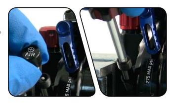
Use a Schrader valve tool to remove the IFP reservoir valve cap.
