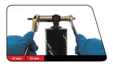
Reinstall the push pin onto the threaded rod and hand thread it along the rod until it rests against the bushing pin (inside the shock eyelet bushing).
