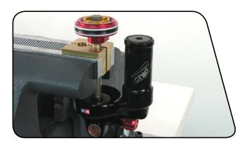
10 Remove and replace the glide ring located on the main piston.
