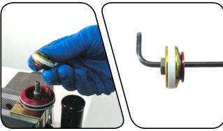
Pull up on the seal head/air piston to remove it from the damper shaft.
