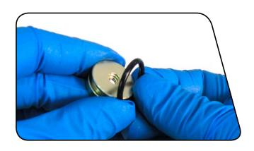
Press the IFP, with the flat side facing out, into the non-threaded side of the reservoir.
