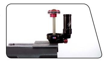
2 Use your finger to push the IFP reservoir cap into the reservoir until it stops.
