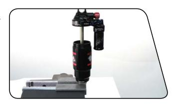
Pour 0.3 mL of Maxima® Maxum4 Extra 15w50 lube into the air can.
