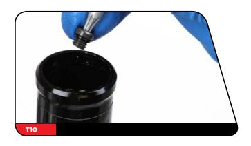
Pour additional suspension fluid into the reservoir until it is level with the top of the reservoir.
