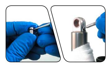
Use your fingers to remove and replace the seal head/air piston quad ring seal and glide rings. Apply a small amout of Parker® O-Lube to the new seals.
