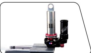
**9** Pour additional RockShox 3 wt suspension fluid into the reservoir until it is level with the top of the reservoir.
