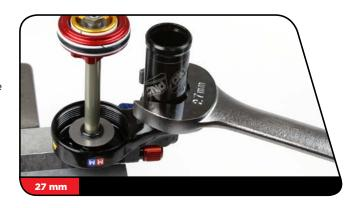
If the compression assembly is still installed in the shock body, use your fingers to pull on the piston nut while rocking it from side to side to remove the compression assembly from the shock body.
