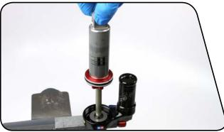
Use a T10 TORX  $^{\circ}$  to reinstall the IFP bleed screw into the IFP. The bleed screw should be submerged in oil.
