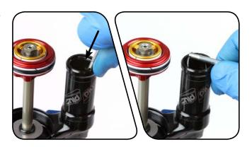
Thread the shock pump into the Monarch air fill adapter, then thread the adapter into the IFP reservoir cap. Pull up on the pump to remove the cap from the reservoir. Unthread the reservoir cap from the adapter and set it aside.
