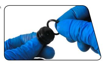
**6** Use a 27 mm open end wrench to unthread the reservoir from the shock body.
