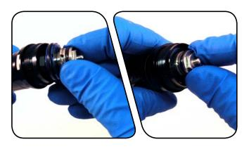
Thread the reservoir into the shock by hand. Use a torque wrench with a 27 mm crowfoot socket to tighten the reservoir to 8.4 N·m (75 in-lb).
