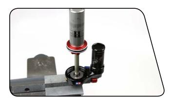
Use the Schrader valve tool to install a new Schrader valve into the reservoir top cap.
