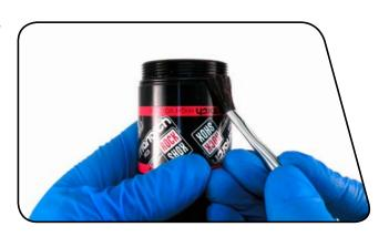
Apply a small amount of blue threadlock to the air can threads.
