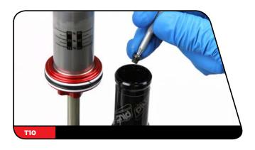
Use a T10 TORX to remove the damper body bleed screw from the damper body eyelet.
