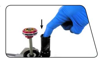
Use the Schrader valve tool to pry the retaining ring out of the groove in the IFP reservoir.
