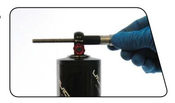
Thead the large end of the catcher onto the rod from the opposite side of the shock eyelet until the rod rests against the shock eyelet.
