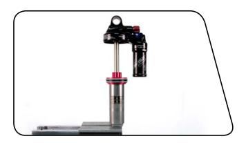
Use a 17 mm open end wrench to loosen and remove the seal head/air piston assembly from the damper body.
