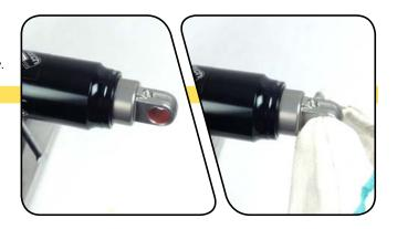
Use a strap wrench to remove the air can. Wrap the strap around the section of the air can furthest from the air can eyelet. Turn the wrench counter-clockwise to unthread the air can.
