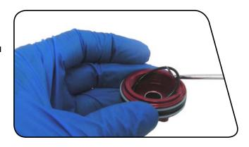
Install the seal head/air piston onto the damper shaft with the seal head threads oriented upward.
