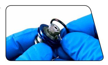
9 Use your fingers to remove the o-ring located at the base of the threads inside the shaft eyelet.
