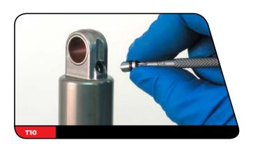
Use a pick to remove the o-ring on the bleed screw. Apply Parker® O-Lube to the new o-ring and reinstall the bleed screw.
