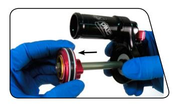
Install the seal head/air piston onto the damper body. While holding only the seal head/air piston, thread it completely onto the damper body.
