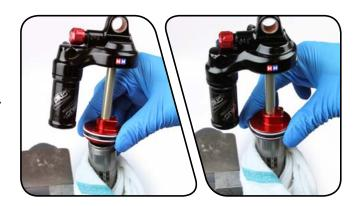
Use a torque wrench with a 17 mm crowfoot socket to tighten the seal head/air piston to 28.2 N·m (250 in-lb).
