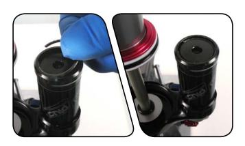
Thread the Monarch air fill adapter/shock pump into the reservoir top cap. Pull up on the pump until the top cap rests against the retaining ring.
