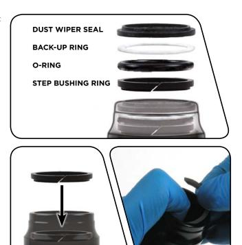
Apply a small amount of Parker® O-Lube grease to the air can o-ring. Install it into the second deepest gland, so that it rests on top of the step bushing.
