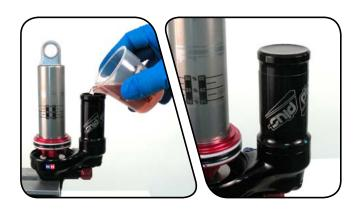
Slowly pull up on the damper body until it stops. This will cycle fluid from the reservoir back into the damper body and purge air bubbles from the system.
