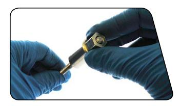
Insert the threaded rod through the bushing pin then through the shock eyelet so that the bushing pin is positioned between the push pin and the shock eyelet.
