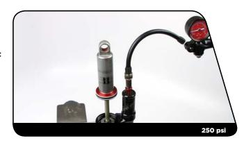
Use a Schrader valve tool to install the reservoir valve cap.
