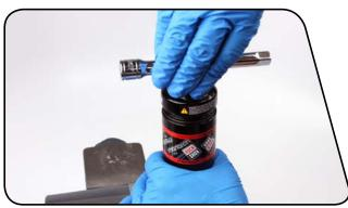
Stabilize the air can with a strap wrench to prevent it from rotating. Use a torque wrench with a 13 mm crowfoot socket to tighten the air can to 16.9 N·m (150 in-lb).
