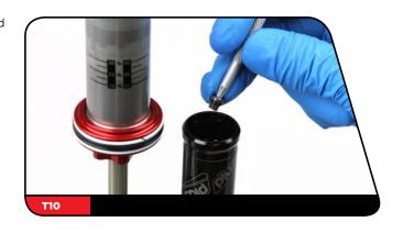
Remove the shock from the vise. Pour the remaining fluid out of the reservoir, then wipe out the reservoir with a clean rag.
