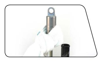
Slowly push down on the damper body to purge air bubbles through the blood part in the slowly start in the through the bleed port in the damper body eyelet. Once there are no more air bubbles, stop pushing on the damper body. Reinstall the damper body bleed screw.
