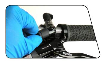
Shortening the hose introduces air into the system. It is necessary to bleed the remote assembly for optimal performance. See the next section, "XLoc Bleed Procedure" for instructions.
