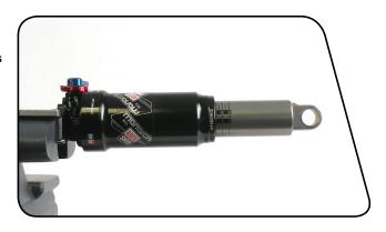
6 If the shock is collapsed so that a minimal amount of damper body is visible, there is still air pressure in the air can. Insert a rag through the damper body eyelet. This will prevent the air can from forcefully ejecting from the shock upon disassembly.
