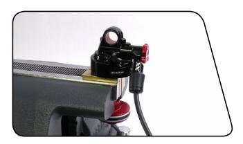
Use a 13 mm open end wrench to loosen the eyelet.
