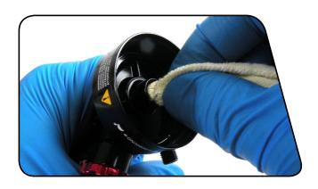
Turn the rebound adjuster counter-clockwise until it stops.
