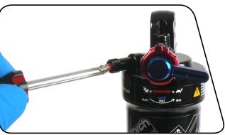
Use a Schrader valve tool to remove the air/nitrogen port cap. Use a small hex wrench or pick to depress the Schrader valve and release all air/nitrogen pressure from the damper. Once the pressure has been released, depress the Schrader valve a second time. If the Schrader valve is able to move, the shock has been completely depressurized.
