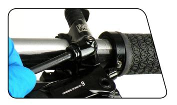
**9** While holding the hose in place, slide the compression fitting and compression nut against the XLoc.
