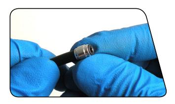
**8** Push the hose firmly into the XLoc until it stops.
