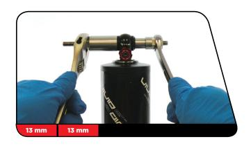
Unthread the catcher from the threaded rod. Remove the tool from the shock eyelet and discard the old bushing.
