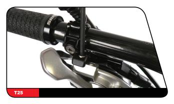
Use a T25 TORX wrench to loosen and remove the XLoc handlebar clamp bolt. Remove the XLoc from the handlebar.
