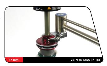
Allow air bubbles to escape from the bleed port in the seal head. Insert the new compression ball into the bleed port.
