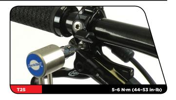
Attach the XLoc shifter to the XLoc bracket with the shifter mounting bolt. Use a T25 TORX® to tighten the shifter mounting bolt to 2.8-3.4 N·m (25-30 in-lb).
