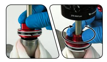
Use a torque wrench with 17 mm crow foot to tighten the seal head/air piston to 28 N·m (250 in-lb).
