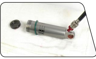
2 Spray isopropyl alcohol on the inside and outside of the damper body and wipe it with a clean rag. Remove a glove and use your finger to inspect the inside and outside of the damper body for scratches, dents, or other surface deformations. If any deformations are found, the damper body will need to be replaced.
