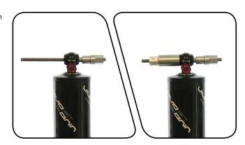
Clamp the catcher in a vise or hold it secure with a 13 mm open end or adjustable wrench.
