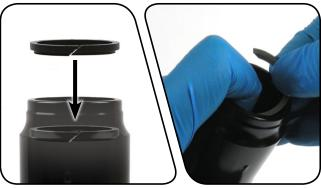
Apply a small amount of Parker® O-Lube grease to the air can o-ring. Install it into the second deepest gland, so that it rests on top of the step bushing.
