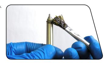
Install the seal head/air piston onto the damper shaft with the seal head threads oriented downward.
