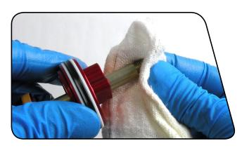
12 Install the topout o-ring and washer onto the shaft.
