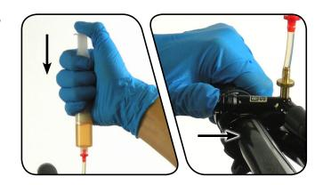
Repeat steps 12-14 until air bubbles no longer move into the suspension fluid. It can take several repetitions of this process to fully void the system of air.
