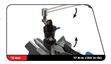
Use a Schrader valve tool to install a new valve core into the valve body.
