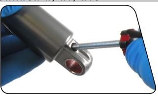
2 Clamp the damper body eyelet into the vise, so the damper body is vertical. Wrap a clean rag around the damper body.
