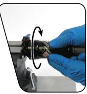
Remove the shock from the vise. Turn the shock over and clamp the damper eyelet into the vise, so the shock is vertical.
