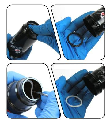
Spray isopropyl alcohol inside the air can and wipe it with a clean rag. Remove a glove and use your finger to inspect the inside and outside of the air can for scratches, dents, or other surface deformations. Replace the air can if it is scratched or damaged.
