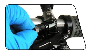
While continuing to push the hose into the XLoc, use a torque wrench with an 8 mm flare nut crowfoot to tighten the compression nut to 5 N·m (47 in-lb).
