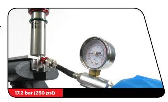
Use a Schrader valve tool to reinstall the air fill port cap.
