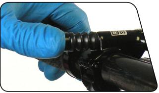
While holding the new hose firmly, use a T10 TORX\* to thread the hose barb into one end of the hose until it bottoms out.
