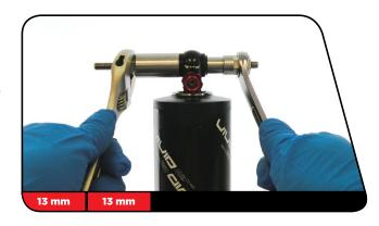
Reinstall the push pin onto the threaded rod and hand thread it along the rod until it rests against the bushing pin (inside the shock eyelet bushing) again.
