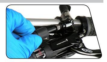
2 Use an 8 mm flare nut wrench to unthread the compression nut.
