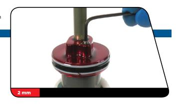
9 Remove the shock and vise blocks from the vise. Use a shock pump with the Monarch air fill adapter to pressurize the damper body to 34.4 bar (500 psi).
