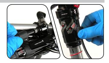
Use an 8 mm flare nut wrench to unthread the compression nuts from the XLoc and the shock swivel fitting.
