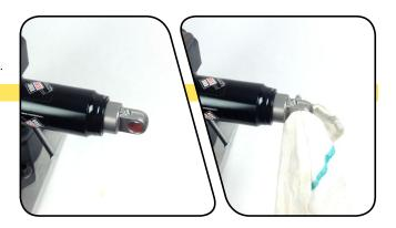
Use a strap wrench to remove the air can. Wrap the strap around the section of the air can furthest from the air can eyelet. Turn the wrench counter-clockwise to loosen and unthread the air can. Once it is completely unthreaded, slowly pull the air can along the shock damper body to remove it.
