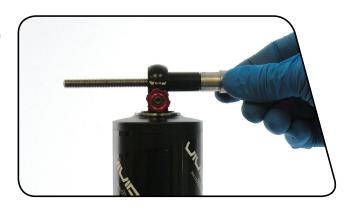
Thread the large end of the catcher onto the rod from the opposite side of the shock eyelet until the rod rests against the shock eyelet.
