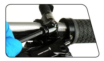
While holding the hose in place, slide the compression fitting and compression nut up to the XLoc.
