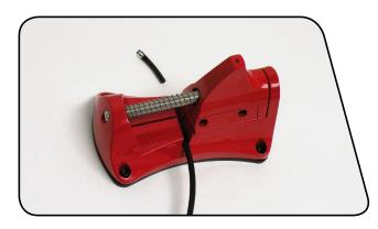
**5** Apply grease to the compression fitting outer surfaces and compression nut threads.
