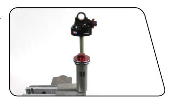
Use a 2 mm hex to unthread and remove the bleed screw, located in the seal head/fixed air piston.
