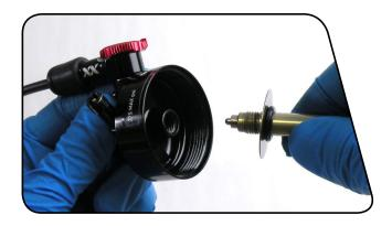
**5** Remove the topout washer and o-ring from the shaft.
