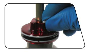
8 Use a 2 mm hex to gently thread the bleed screw into the bleed port until you feel it touch the compression ball. Tighten the bleed screw an additional ½ turn.
