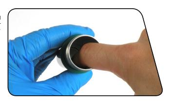
Remove the IFP o-ring. Spray the IFP with isopropyl alcohol and wipe it with a clean rag. Apply a small amount of grease to the new o-ring and install it.
