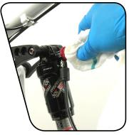
Hold the XLoc button in the extended (locked) position and pull out the syringe plunger. Small bubbles will move into the suspension fluid as air is pulled from the system.
