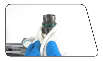
Pour new RockShox 7wt suspension fluid into the the damper body until it is level with the top of the damper body. Use your finger to remove any bubbles from the surface of the fluid.
