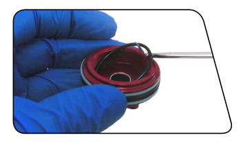
Install the seal head/air piston onto the damper shaft with the seal head threads oriented upward.
