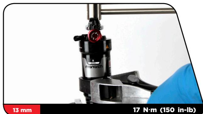
**7** Use a Schrader valve tool to install a new Schrader valve into the air can valve.
