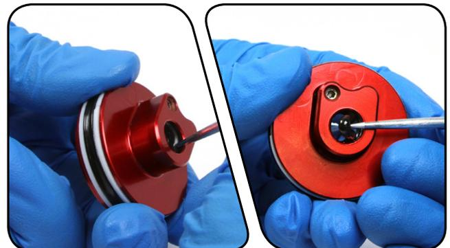
**7** Use a pick to remove the inner o-ring, located at the base of the threads in the seal head/air piston.
