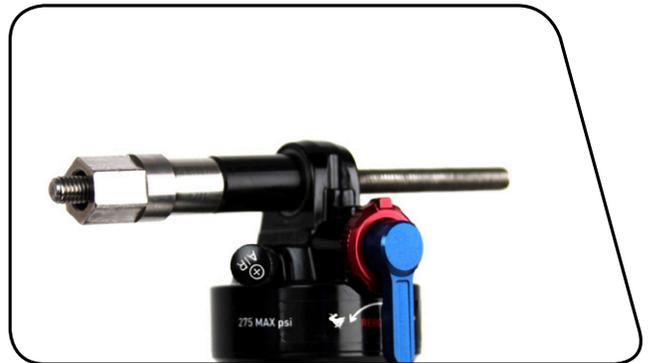
**3** Thread the large, open end of the catcher onto the rod until it rests on the eyelet.
