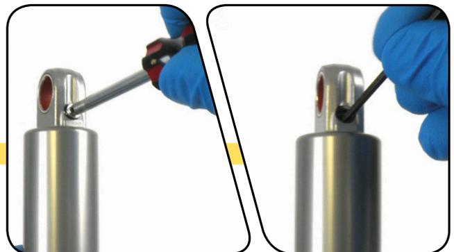
**4** Use a Schrader valve tool to remove the valve core.
