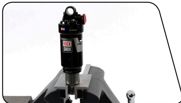
**6** Stabilize the air can with a strap wrench to prevent it from rotating. Use a torque wrench with a 13 mm crowfoot socket to tighten the air can to 17 N·m (150 in-lb).
