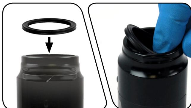
**7** Install the air can back-up ring into the same gland, so that it rests between the quad ring and the top of the gland.
