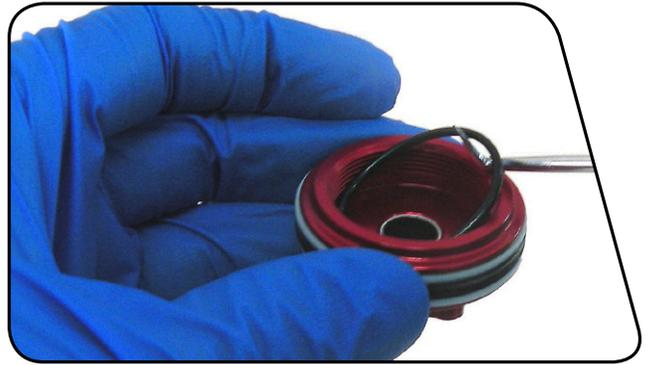
**8** Install the seal head/air piston onto the damper shaft with the seal head threads oriented upward.
