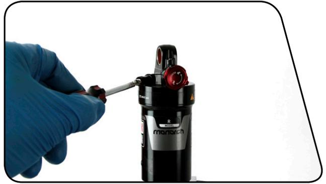
**8** Use a shock pump to inflate the shock to the desired air pressure, then install the valve cap.
