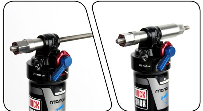
**3** Clamp the catcher in a vise or hold it secure with a 13 mm open end or adjustable wrench.
