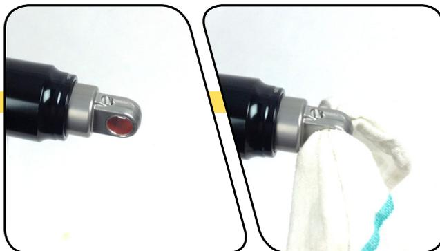
**7** Use a strap wrench to remove the air can. Wrap the strap around the section of the air can furthest from the shaft eyelet. Turn the wrench counter-clockwise to loosen and unthread the air can.
