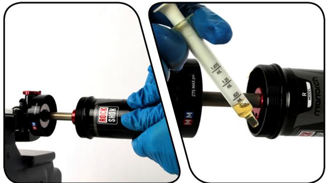
**4** Continue to press the air can onto the damper body until the air can threads and shaft eyelet threads make contact. Thread the air can clockwise into the shaft eyelet. Tighten the air can, by hand, into the shaft eyelet.
