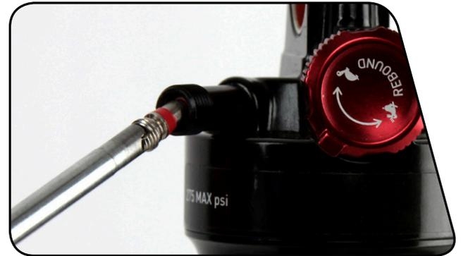
**3** Use a Schrader valve tool to remove the air/nitrogen port cap.
