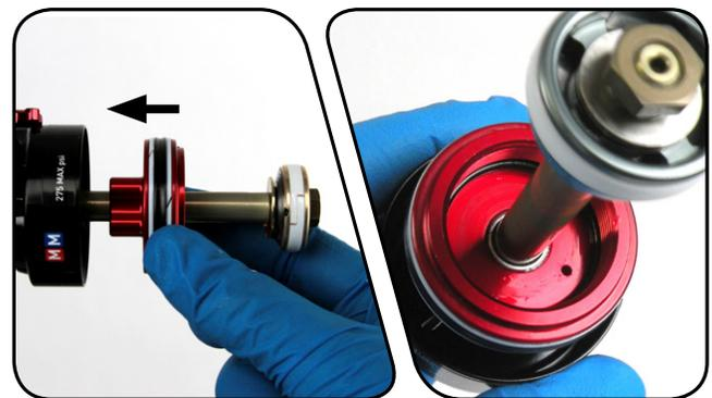
**7** Use a pick or 1.5 mm hex wrench to push and remove the compression ball out of the backside of the seal head through the bleed port.
