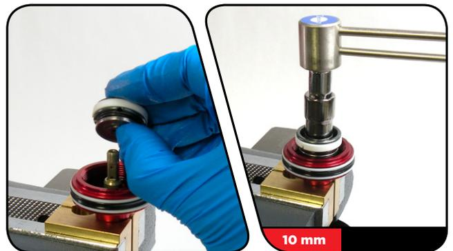
**10** Remove the shaft assembly from the vise and set it aside.
