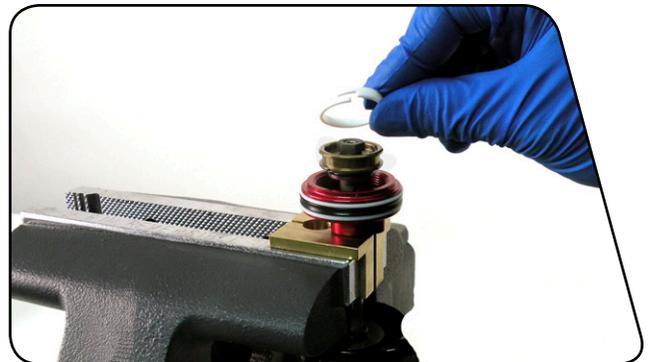
**4** Use a 10 mm wrench to unthread the piston nut. Remove the main piston assembly.
