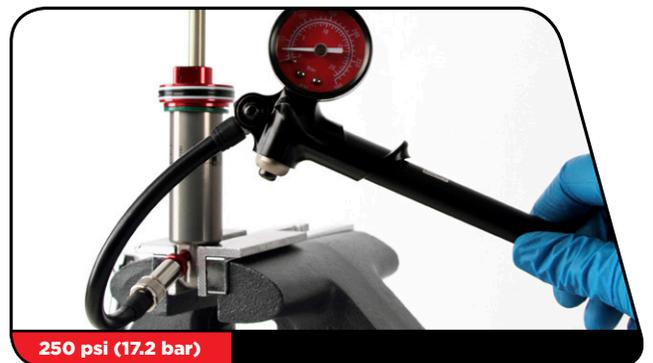
**10** Use a Schrader valve tool to install the damper air fill port cap.
