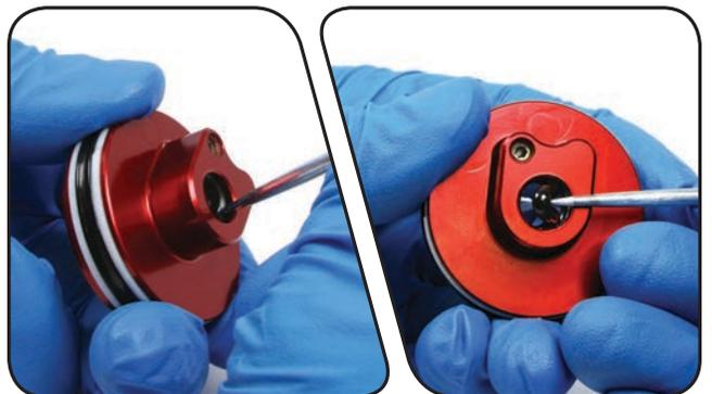
**8** Use a pick to remove the inner o-ring, located at the base of the threads in the seal head/air piston.
