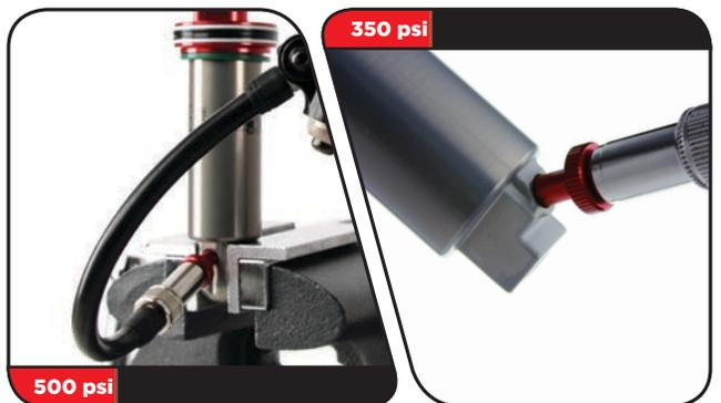
**10** Use a Schrader valve tool to install the air fill port cap.
