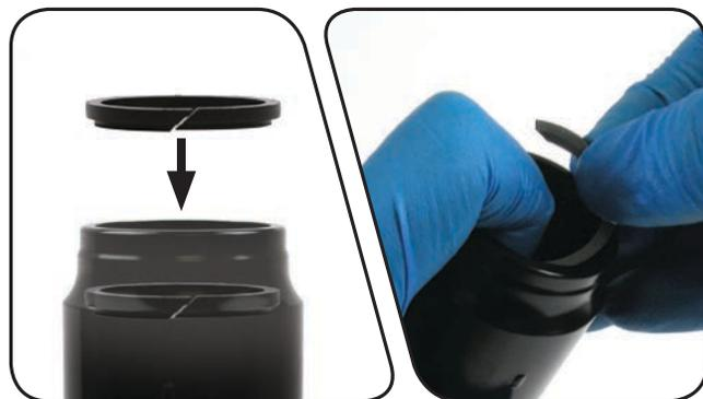
**6** Replace the air can o-ring with the quad ring from the seal kit. Apply a small amount of Parker® O-Lube grease and install it into the second deepest gland, so that it rests on top of the step bushing.
