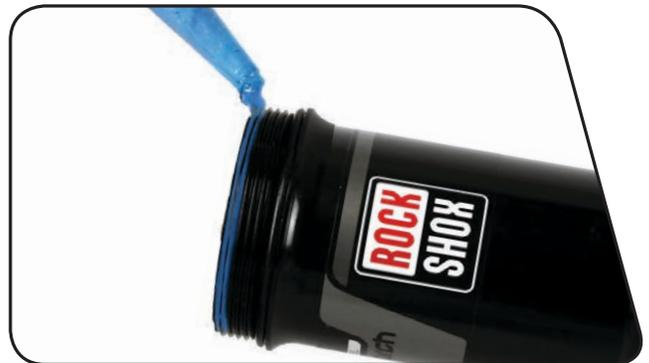
**3** Position the threaded side of the air can over the damper body eyelet. Firmly press the air can onto the air piston and damper body until the air can is approximately 30 mm from the shaft eyelet threads. Pour/inject 0.3 mL of Maxima® Maxum4 Extra 15w 50 into the air can.
