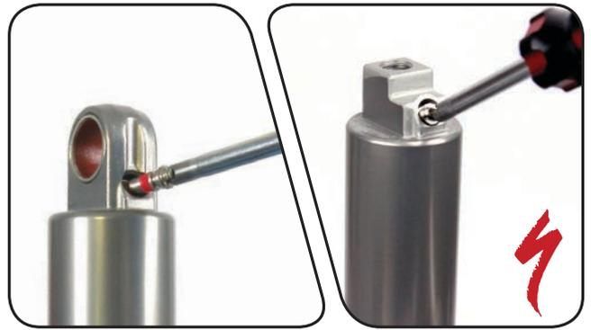
**5** Clamp the shaft eyelet into a bench vise, with the shock positioned horizontally.
