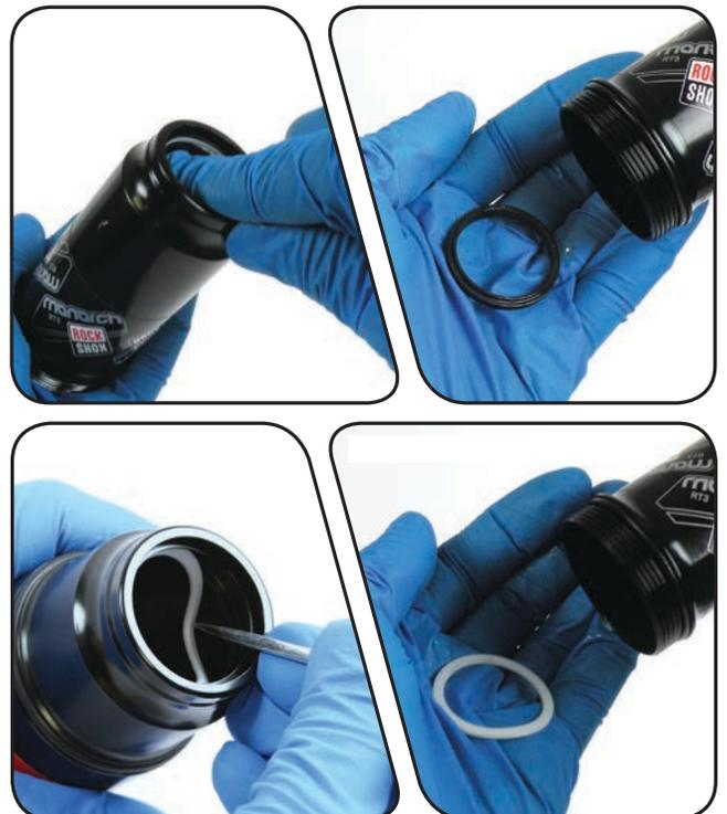
**4** Spray isopropyl alcohol inside the air can and wipe it with a clean rag. Remove a glove and use your finger to inspect the inside and outside of the air can for scratches, dents, or other surface deformations. Replace the air can if it is scratched or damaged.
