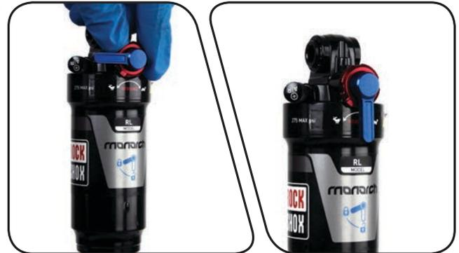
**2** Check and record your current air pressure setting to assist with post-service set up.
