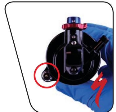
**7** Use a Schrader valve tool to install a new Schrader valve into the air can valve.
