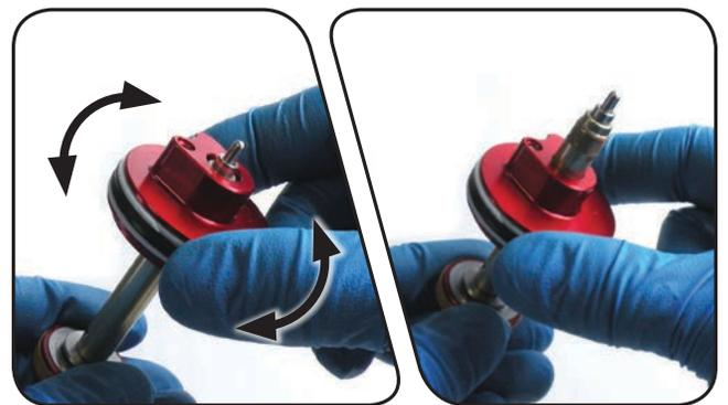
**11** Use isopropyl alcohol and a rag to clean the grease from the shaft threads.
