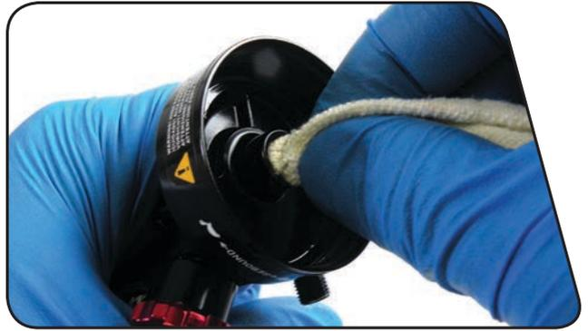
**15** Turn the rebound adjuster counter-clockwise until it stops.
