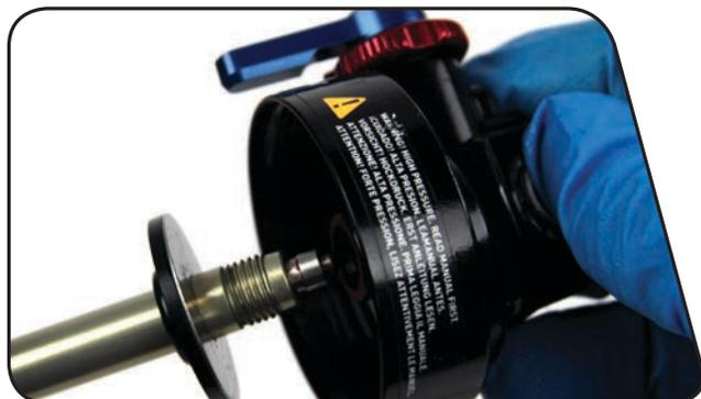
**5** Remove the bottom out washers and o-ring from the shaft.
