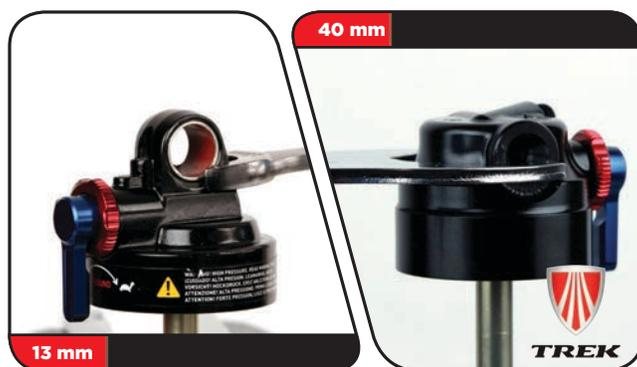
**4** Remove the shaft assembly from the vise. Unthread the shaft from the eyelet by hand.
