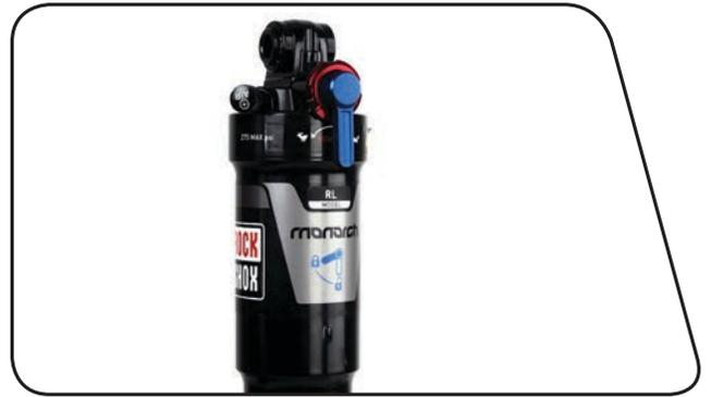
**6** Stabilize the air can with a strap wrench to prevent it from rotating. Use a torque wrench with a 13 mm (Trek®: 40mm) crowfoot socket to tighten the air can to 17 N·m (150 in-lb).
