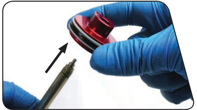
**7** Use a pick to remove the o-ring located in the interior of the seal head.
