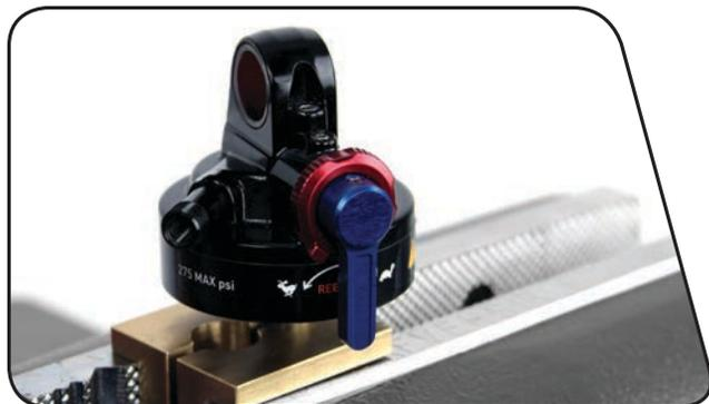
**3** Use a 13 mm (Trek®: 40 mm) open end wrench to loosen the eyelet.
