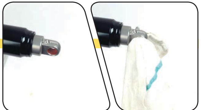
**7** Use a strap wrench to remove the air can. Wrap the strap around the section of the air can furthest from the air can eyelet. Turn the wrench counter-clockwise to loosen and unthread the air can.
