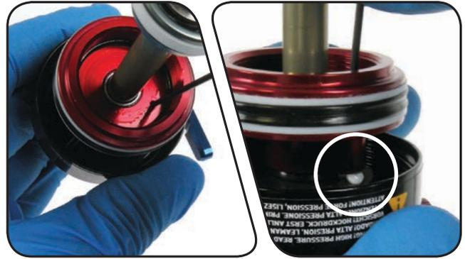
**8** Spray the entire shaft and piston assembly with isopropyl alcohol and wipe it with a clean rag.
