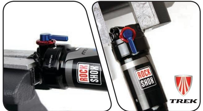
**6** If the shock is collapsed so that a minimal amount of damper body is visible, there is still air pressure in the air can. Insert a rag through the damper body eyelet. This will prevent the air can from forcefully ejecting from the shock upon disassembly.
