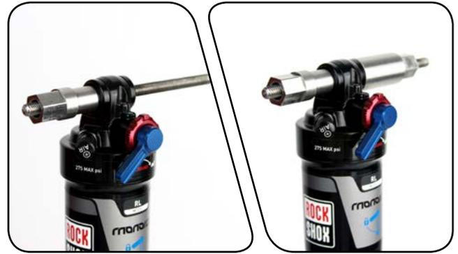
**3** Clamp the catcher in a bench vise or hold it secure with a 13 mm open end or adjustable wrench.
