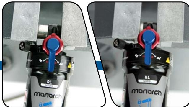
**6** Continue to press the eyelet bushing until it is seated in the shaft eyelet.
