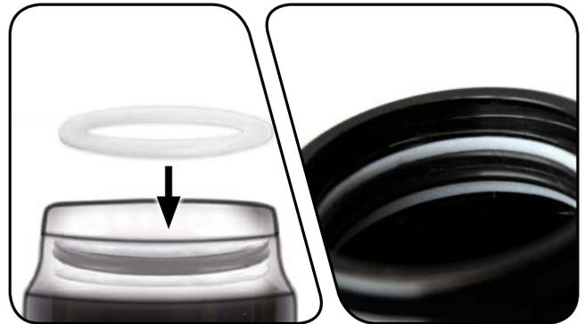
**7** Orient the new dust wiper seal step side up. Install it into the dust wiper seal groove at the top of the air can.
