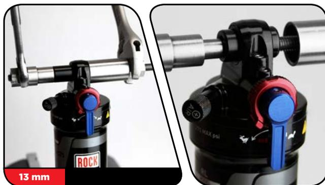
**5** Unthread the catcher from the threaded rod and remove the tool from the shaft eyelet.
