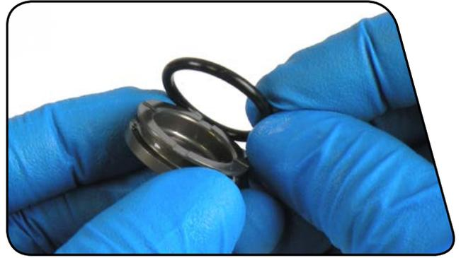
**5** Insert the IFP into the damper body with the stepped side visible. Use a metric caliper or ruler to push the IFP to the depth specified in the table below.
