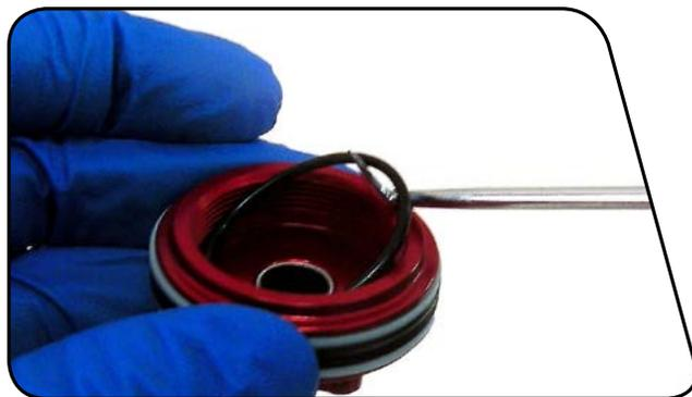
**10** Use a pick or 1.5 mm hex wrench to push and remove the compression ball out of the backside of the seal head through the bleed port.
