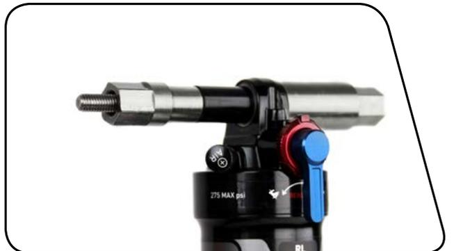
**4** Clamp the catcher in a bench vise or hold it secure with a 13 mm wrench.
