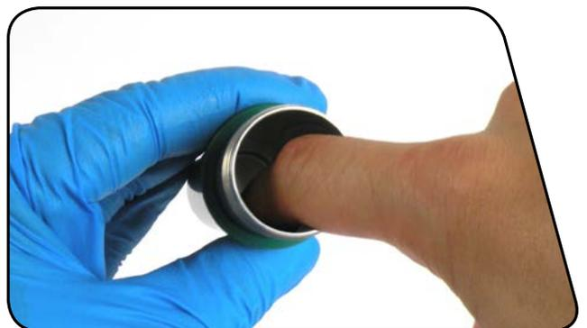
**4** Remove the IFP o-ring. Spray isopropyl alcohol on the IFP o-ring and clean it with a rag.
