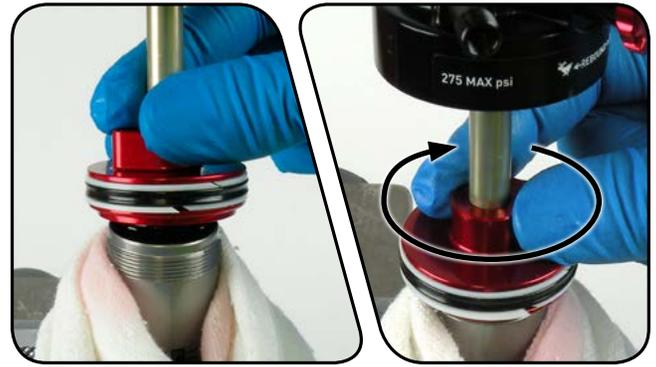
**5** Use a torque wrench with 17 mm crow foot to tighten the seal head/air piston to 28 N·m (250 in-lb).
