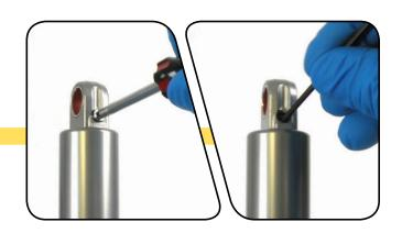
4 Use a Schrader valve tool to remove the valve core.
