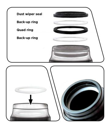
**5** Apply a small amount of Parker® O-Lube grease to the new quadring and install it above the back-up ring in the second deepest gland.
