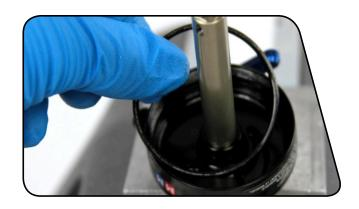
Reinstall the seal head/air piston onto the damper shaft with the seal head threads oriented upward.
