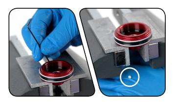
Remove the bottom out washer and o-ring from the shaft.
