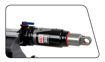
6 If the shock is collapsed so that a minimal amount of damper body is visible, there is still air pressure in the air can.
