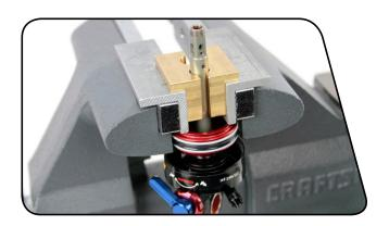
Use a small Torx® wrench or pick to reinstall the shim stack on one side of the main piston. Use your fingers to squeeze the shims and center the shim stack.
