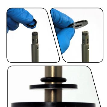
Use a pick to remove the o-ring located in the interior of the shaft eyelet threads.
