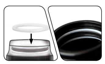
Orient the new dust wiper seal step side up. Install it into the dust wiper seal gland at the top of the air can.
