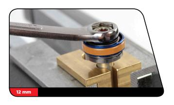
$\hbox{\bf 5} \hbox{ Remove the main piston assembly by using a small torx} \hbox{\bf @ wrench or pick to slide the main assembly off the shaft.}$
