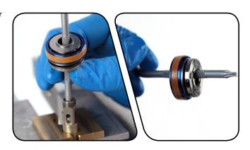
Use a pick to remove the seal head/air piston seal and glide rings.
