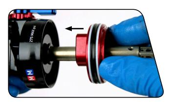
Use the SRAM shaft clamp tool to clamp the seal head/air piston into a vise with the eyelet positioned vertically.
