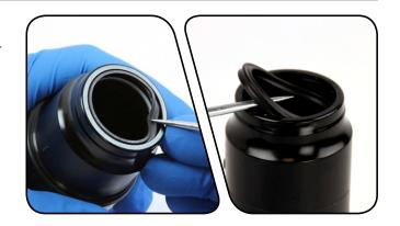
Use a pick to remove the two back-up rings out of the air can.
