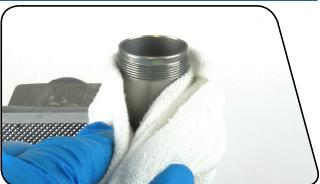
Pour new RockShox 7wt suspension fluid into the the damper body until it is level with the top of the damper body. Use your finger to remove any bubbles from the surface of the fluid.
