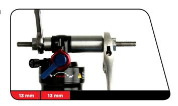
Reinsert the threaded rod and push pin through the shaft eyelet.
