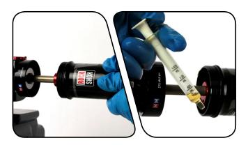
Continue to press the air can onto the damper body until the air can threads and shaft eyelet threads make contact. Thread the air can clockwise into the shaft eyelet. Hand-tighten the air can onto the shaft eyelet.
