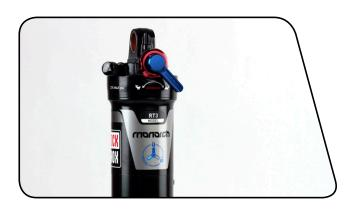
5 Stabilize the air can with a strap wrench to prevent it from rotating. Use a torque wrench with a 13 mm crowfoot socket to tighten the air can to 4.5 N·m (40 in-lb).
