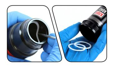
Spray isopropyl alcohol inside the air can and wipe it with a clean rag. Remove a glove and use your finger to inspect the inside and outside of the air can for scratches, dents, or other surface deformations. Replace the air can if it is scratched or damaged.
