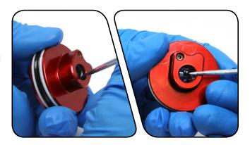
**9** Use a pick to remove the inner o-ring, located at the base of the threads in the seal head/air piston.
