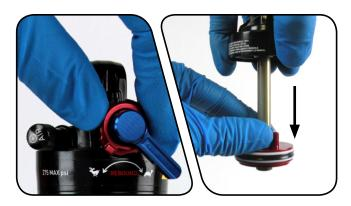
Install the seal head/air piston onto the damper body and thread it completely onto the damper body.
