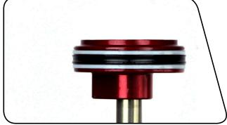
Pull on the seal head/air piston to remove it from the damper shaft.
