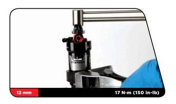
Use a Schrader valve tool to install a new Schrader valve into the air can valve.
