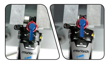
6 Continue to press the eyelet bushing until it is seated in the shaft eyelet.
