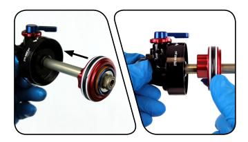
Use the SRAM shaft clamp tool to clamp the seal head/air piston into a vise with the main piston positioned vertically.
