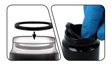
6 Install the other back-up ring by inserting one end into the air can, then push the remainder of the ring into the can, so that it rests on the quad ring at the top of the second deepest gland.
