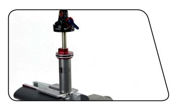
Use a 2 mm hex to unthread and remove the bleed screw, located in the seal head/air piston.
