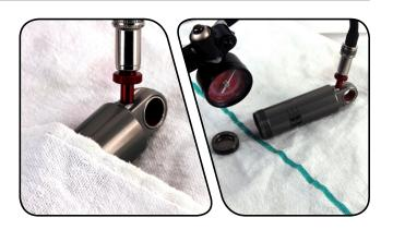
2 Spray isopropyl alcohol on the inside and outside of the damper body and wipe it with a clean rag.
