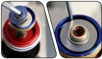
Thread the main piston, by hand, onto the damper shaft. Use a torque wrench with a 12 mm socket to tighten it to 4.5 N·m (40 in-lb).
