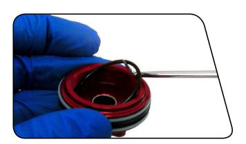
Use a pick or 1.5 mm hex wrench to push and remove the compression ball out of the backside of the seal head through the bleed port.
