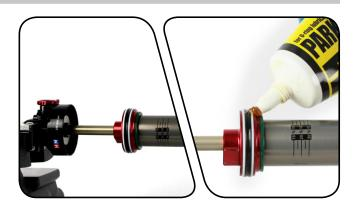
2 Apply a small amount of grease to the air can threads. Position the threaded side of the air can over the damper body eyelet.
