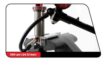
10 Use a Schrader valve tool to install the air fill port cap.
