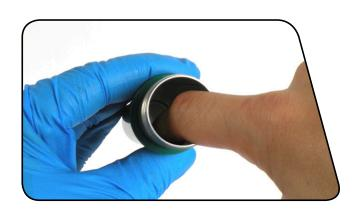
Remove the IFP o-ring. Spray the IFP with isopropyl alcohol and wipe it with a clean rag.
