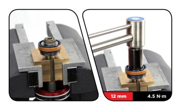
17 Remove the shaft assembly from the vise and set it aside.
