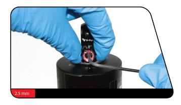
Insert the tips of the pin spanner into the holes in the lock ring.
