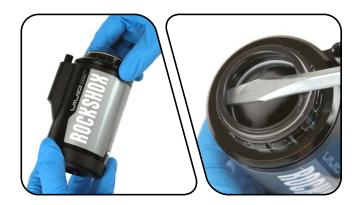
Place a new dust wiper seal onto the end of a seal press tool as shown. Use the seal press tool to install the dust wiper seal into the smaller opening of the air can collar until there is no gap between the dust wiper seal and the air can collar.
