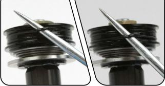
5 Use a socket wrench with a 10 mm socket to unthread the piston nut. Insert a 2 mm hex wrench through the piston nut and into the piston bolt, main piston, and shim stack washers. Keeping all parts together, carefully remove the piston assembly and hex wrench from the shaft and set it aside.
