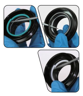
Use a pick to remove and replace the o-ring located just below the threads on the outside of the air can collar. Spray isopropyl alcohol on the air can collar and clean it with a rag.
