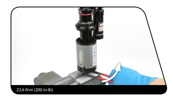
Clamp the RockShox Vivid Air Can Wrench into the vise and place the air can into it. Push the air can collar down the damper body and thread it into the air can.
