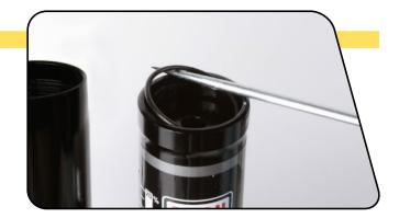
Thread the Vivid Pump Adapter into a shock pump. Thread the pump and Vivid Pump Adapter into the IFP reservoir cap. Pull up on the pump and rock it side to side to remove the reservoir cap from the IFP reservoir. Remove the reservoir cap assembly from the pump/adapter.
