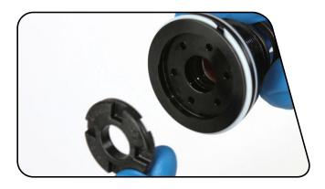
Remove and replace the two seal head glide rings and the quad seal.
