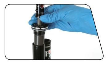
Remove the shock from the vise and pour the fluid from the damper body into an oil pan.
