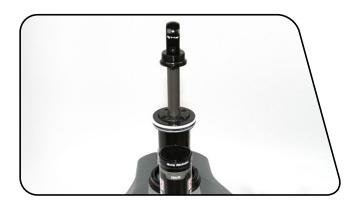
Recall the number from the top of the air can that you recorded. This will assist you with the proper alignment of the air can relative to the Beginning Stroke Rebound knob.
