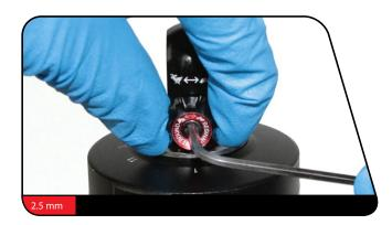
Use a 2.5 mm hex wrench to turn the bolt clockwise to install the Beginning Stroke Rebound knob.
