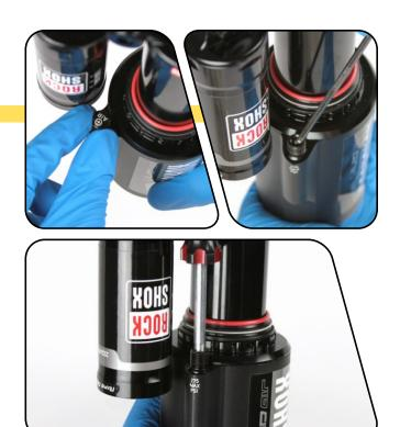
Use a T10 TORX<sup>®</sup> wrench to remove the IFP reservoir fill cap. Use a small hex wrench or pick to depress the Schrader valve and release all air pressure from the IFP reservoir.
