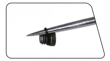
Use a T10 TORX<sup>®</sup> wrench to remove the IFP bleed screw.
