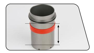
Remove and replace the air can o-ring, located inside the large opening of the air can, just above the internal threads.
