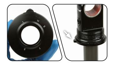
Pour 3 cc of Maxima<sup>®</sup> Maxum 4 Extra 15w50 oil into the air can inner sleeve. Rotate the air can to spread the oil evenly on the inner surface of the sleeve.
