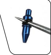
Use your fingers to push the compression needle into the compression valve as shown.
