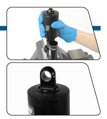
Spray isopropyl alcohol on the air can lock ring threads and shaft eyelet threads and clean them with a rag. Apply red threadlock to the lock ring threads. Install the lock ring over the shaft eyelet, then use the pin spanner to continue to turn the lock ring just until it starts to tighten. Remove the shock from the vise.
