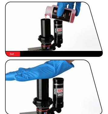
12 Once most of the fluid from the damper body has moved to the reservoir, use the palm of your hand to tap downward on the top of the reservoir repeatedly to move fluid back into the damper body. This will further assist in purging air bubbles from the system.
