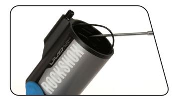
Use a pick to remove the air can inner sleeve centering ring from the bottom of the air can.
