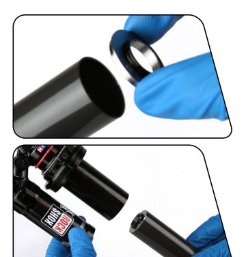
Clamp the body eyelet into the vise. Install the air can centering ring onto the air can collar with the chamfered, stepped side facing upward.
