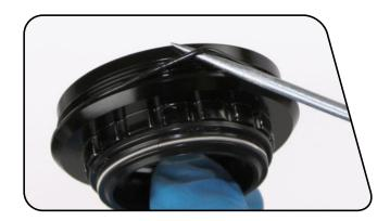
Install a new white back-up ring, quad seal, and blue back-up ring, stepped side oriented upward, into the threaded side of the air can air can collar.
