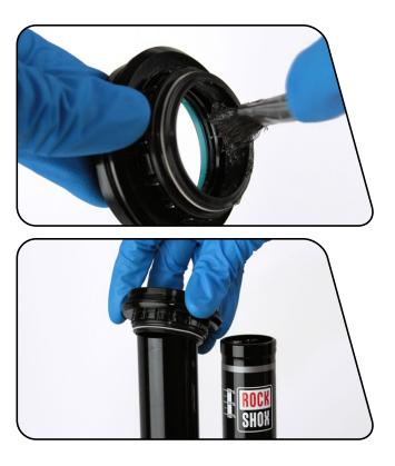
Remove and replace the crush washer on the damper tube centering ring.
