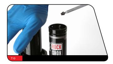
Pour additional fluid into the damper body until the fluid is level with the top of the threads.
