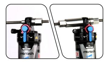
Clamp the catcher in a vise or hold it secure with a 13 mm wrench. Use a second 13 mm wrench to thread the push pin along the rod until the push pin pushes the eyelet bushing out of the eyelet.
