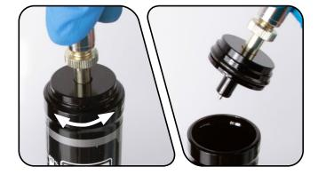
Remove and replace the IFP reservoir cap o-ring.
