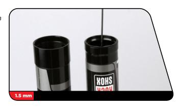
Remove and replace the crush washer on the damper tube centering ring.
