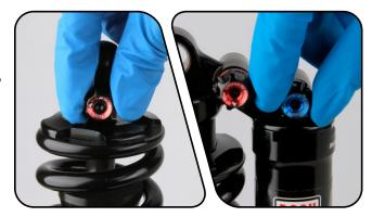
**2** Turn the Preload Adjuster counter-clockwise until it stops.
