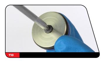
Remove and replace the IFP bleed screw o-ring.
