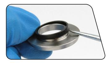
Place the damper tube centering ring onto the end of the damper tube that does not have holes. Hold the shock with the damper body opening facing downward. Insert the damper tube into the damper body and rotate it until the centering ring is seated in its groove.
