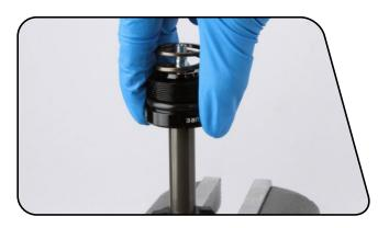
Remove the bottom out bumper from the shaft. Clean and inspect the shaft for damage and replace if necessary.
