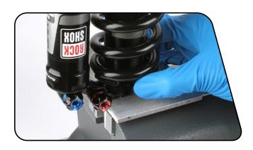
Remove the spring retainer and spring.
