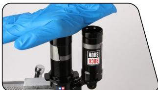
Once most of the fluid from the damper body has moved to the reservoir, use the palm of your hand to tap downward on the top of the reservoir repeatedly to move fluid back into the damper body. This will further assist in purging air bubbles from the system.
