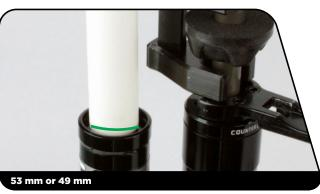
Use a T10 TORX<sup>®</sup> wrench to install the bleed screw into the bleed port and tighten it until the IFP begins to spin.
