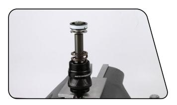
Remove and replace the piston glide ring and the two o-rings located under the glide ring.
