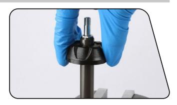
Grease the interior of the seal head and install it onto the shaft assembly with the Counter Measure<sup>TM</sup> Spring oriented upward.
