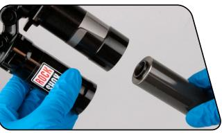
Pour RockShox 3wt suspension fluid into the damper body until it is level with the top of the damper tube. Fluid will begin to bleed into the IFP reservoir.
