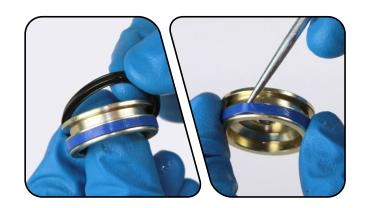
Remove and replace the IFP reservoir o-ring and shoulder washer, located above the threads inside the IFP reservoir.
