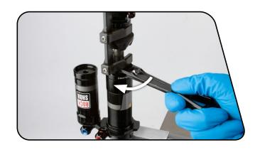
Use a torque wrench inserted into the slot of the spanner wrench to tighten the seal head to 28.2 N·m (250 in-lb).
