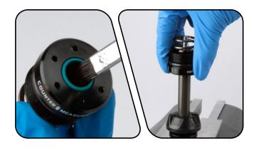
Use the 2 mm hex wrench to install the piston assembly onto the shaft. Use a torque wrench with a 10 mm socket to tighten the nut to 7.9 N·m (70 in-lb).
