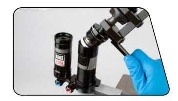
Use the RockShox Vivid 24 mm Spanner Wrench to turn the seal head clockwise and install it into the damper body.
