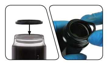
Spray isopropyl alcohol on the air can threads and eyelet body threads and clean them with a rag.
