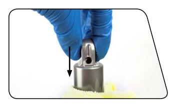
If the damper body is all the way down and air bubbles are still present, then reinstall the damper bleed screw, remove the IFP bleed screw, and repeat steps 9-12 until no more air bubbles are present.
