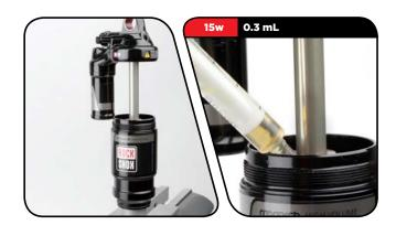
Insert a 5 inch socket extension through the shaft eyelet. Push down on the shaft eyelet while pulling the air can up until the air can threads engage with the eyelet threads.
