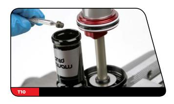
Use a T10 TORX wrench to remove the damper body bleed screw from the damper body eyelet.
