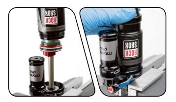
Remove the shock from the vise. Turn it over and clamp the damper body eyelet into the vise.
