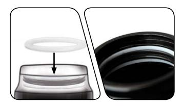
Orient the new dust wiper seal step side up. Install it into the dust wiper seal groove at the top of the air can.
