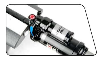
If the shock is collapsed so that a minimal amount of damper body is visible, there is still air pressure in the air can.
