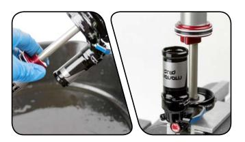
Use the Schrader valve tool to install a new Schrader valve into the IFP reservoir cap.
