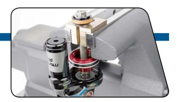
Use a 12 mm socket wrench to remove the main piston nut.
