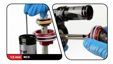
Use your hand to install the seal head/air piston onto the damper
