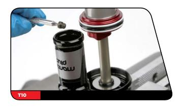
Remove the shock from the vise. Pour the fluid out of the IFP reservoir. Spray isopropyl alcohol in the IFP reservoir and clean it with a rag.
