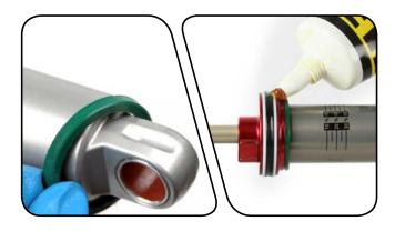
Clamp the shaft eyelet into the vise.
