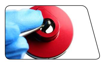
8 Use a pick to remove and replace the inner o-ring, located at the base of the threads in the seal head/air piston.
