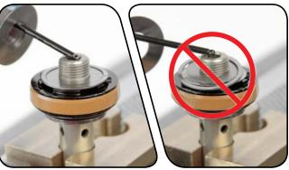
Thread the main piston nut onto the damper shaft. Use a torque wrench with a 12 mm socket to tighten the main piston nut to 4.5 N·m (40 in-lb).
