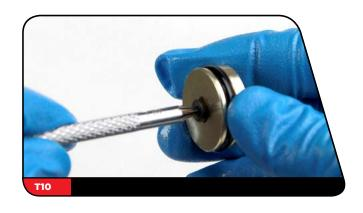
Remove and replace the IFP o-ring.
