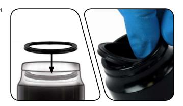
Install the second backup ring by inserting one end into the air can, then push the remainder of the ring into the can, so that it rests on the quad seal at the top of the second deepest groove.
