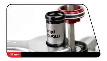
**Monarch Plus™ RC3 Only:** Use your fingers to remove the compression assembly from the IFP reservoir or eyelet.
