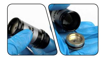
Use a T10 TORX\* wrench to remove the IFP bleed screw. Replace the o-ring on the IFP bleed screw.
