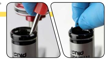
Thread the Monarch™ air vavle adapter tool into a shock pump. Thread the pump and adapter into the IFP reservoir cap. Pull up on the pump and rock it side to side to remove the IFP reservoir cap from the IFP reservoir.
