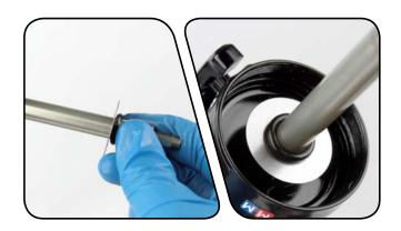
Use your fingers to remove and replace the o-ring located inside the shaft eyelet threads.
