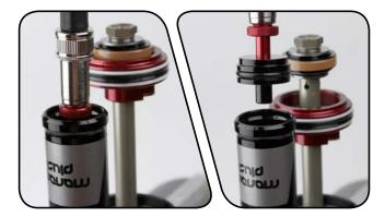
Remove and replace the IFP reservoir cap o-ring.
