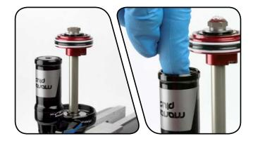
Use a Schrader valve tool to remove the retention clip from the IFP reservoir.
