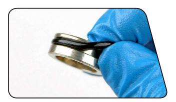
12 Install the IFP, flat side up, into the IFP reservoir. Use a metric caliper or ruler to push the IFP into the reservoir to a depth of 35 mm.
