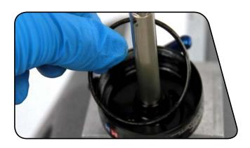
Install the seal head/air piston onto the damper shaft.
