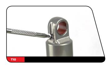
Wrap a clean rag around the damper body. Slowly push down on the damper body to purge the air bubbles from the bleed port in the damper body eyelet.
