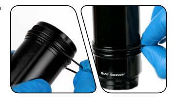
11 High Volume Air Cans: Apply a small amount of suspension specific grease to the inside of the sleeve. This stops the o-rings from rolling as the sleeve slides over them.
