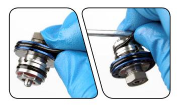
Use your fingers to remove and replace the o-ring located inside the eyelet threads.
