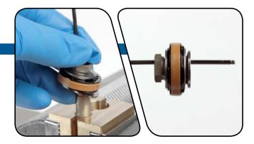
Remove the seal head/air piston from the damper shaft.
