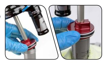
Use a torque wrench with a 17 mm crowfoot to tighten the seal head/air piston to 28 N·m (248 in-lb).
