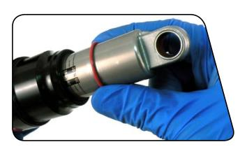
9 Reinstall the shock mounting hardware (see the Mounting Hardware And Bushing Service section).
