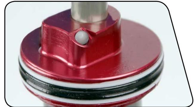
**7** Use a 2 mm hex wrench to thread the bleed screw into the bleed port until you feel it touch the compression ball, then tighten the bleed screw an additional ½ turn.
