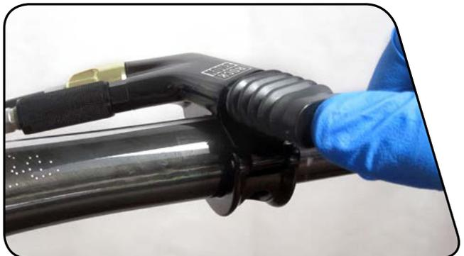
**3** Remove the syringe from the rear shock bleed port.
