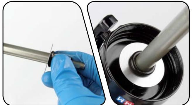
**12** Use your fingers to remove and replace the o-ring located inside the shaft eyelet threads.
