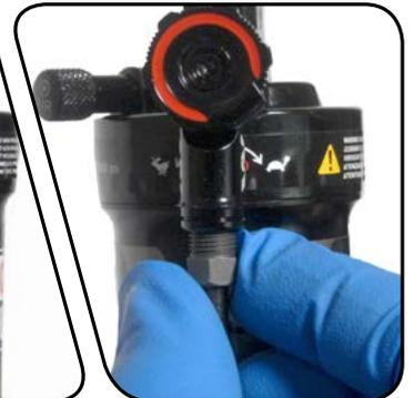
**10** While continuing to push the hose into the rear shock banjo fitting, use a torque wrench with an 8 mm crowfoot socket to tighten the compression nut to 5 N·m (44 in-lb).
