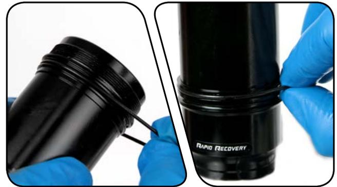
**11 High Volume Air Cans:** Apply a small amount of suspension specific grease to the inside of the sleeve. This stops the o-rings from rolling as the sleeve slides over them.
