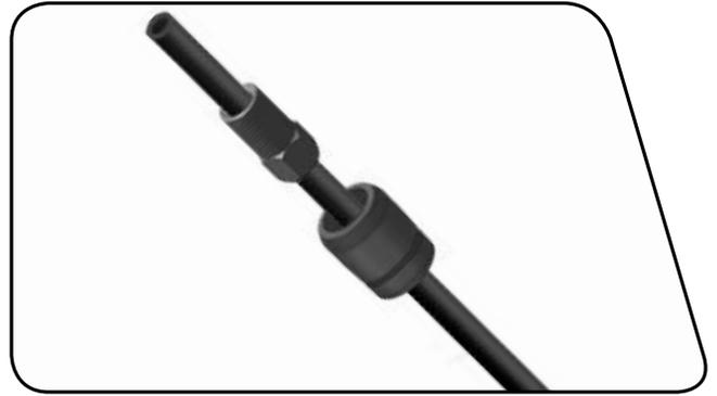
**8** Use an Avid Hydraulic Hose Barb Driver Tool or a T10 TORX® wrench to thread the new hose barb into the end of the hose until it is flush. Install the compression fitting onto the hose.
