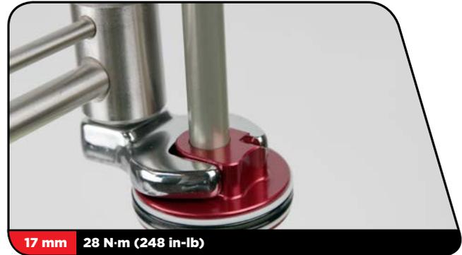
**6** Allow air bubbles to escape from the bleed port in the seal head. Insert the new compression ball into the bleed port.
