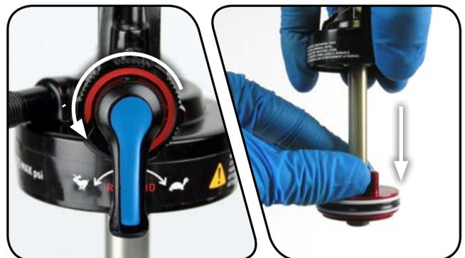
**4** Use your hand to install the seal head/air piston onto the damper body.
