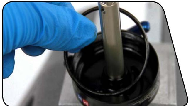
**13** Use your fingers to remove and replace the seal head/air piston seal and glide rings.
