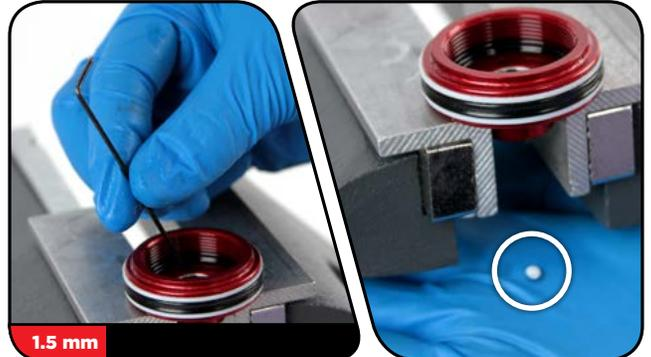
**11** Remove and replace the bottom out washer and o-ring from the shaft.
