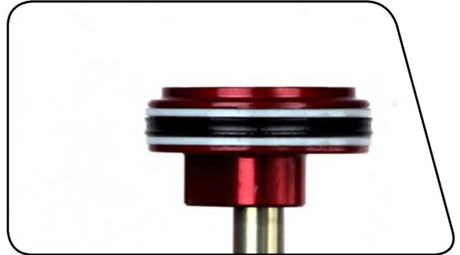
**14** Install the seal head/air piston onto the damper shaft.
