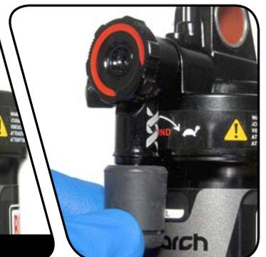
**Cutting the hose introduces air into the system. It is necessary to bleed the remote assembly for optimal performance. See [XLoc Full Sprint™ Bleed Procedure](#) for instructions.**
