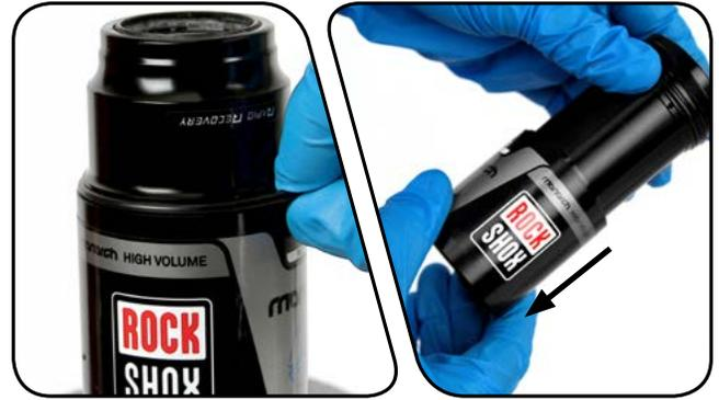
**10 High Volume Air Cans:** Use your fingers to remove and replace the high volume sleeve o-rings.
