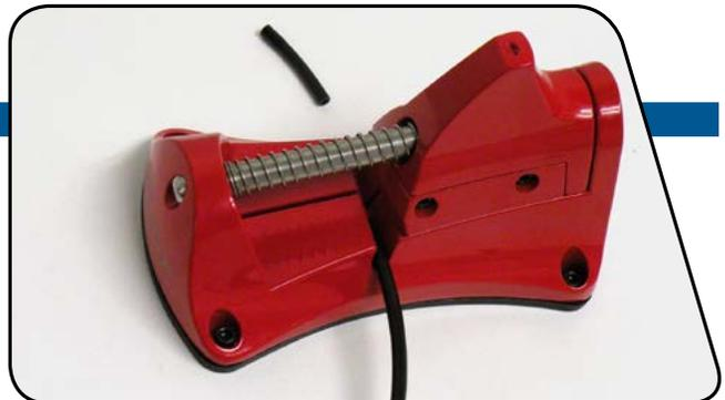
**7** Apply Slick Honey® to the hose barb threads, the new compression fitting outer surfaces, and the compression nut threads.
