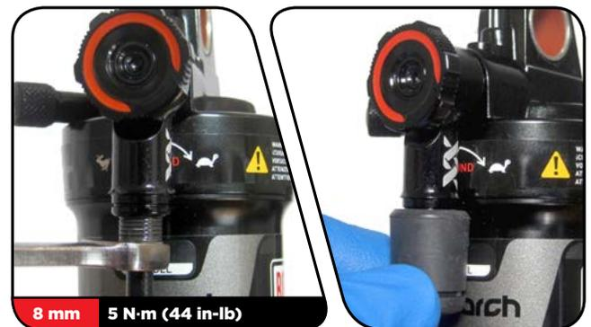
**Shortening the hose introduces air into the system. It is necessary to bleed the remote assembly for optimal performance. See [XLoc Full Sprint™ Bleed Procedure](#) for instructions.**
