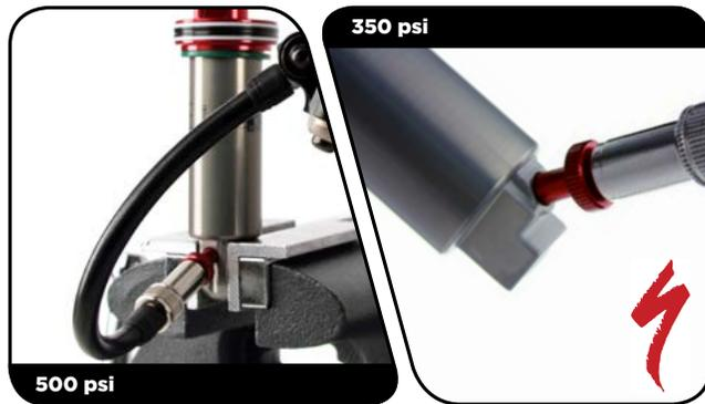
**9** Use a Schrader valve tool to install the damper air/nitrogen fill port cap.
