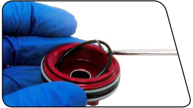
**10** Use a 1.5 mm hex wrench to push the compression ball out of the backside of the seal head through the bleed port.
