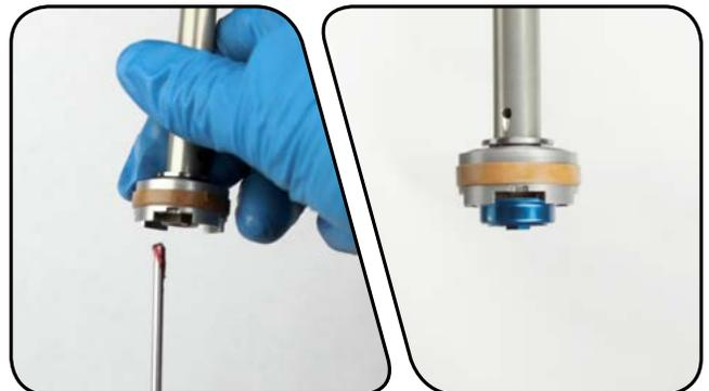
**18** Test the compression rod and top hat function by rotating the compression lever to the closed position and pushing on the top hat. The top hat should have a small amount of movement. If it does not move, adjust the top hat spring so it is seated inside the groove.
