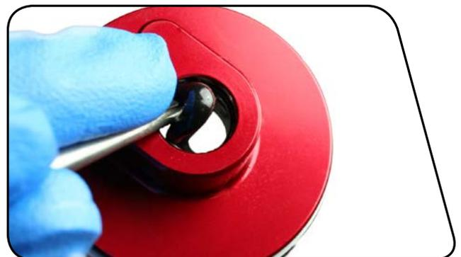
**9** Use a pick to remove and replace the inner o-ring, located at the base of the threads in the seal head/air piston.
