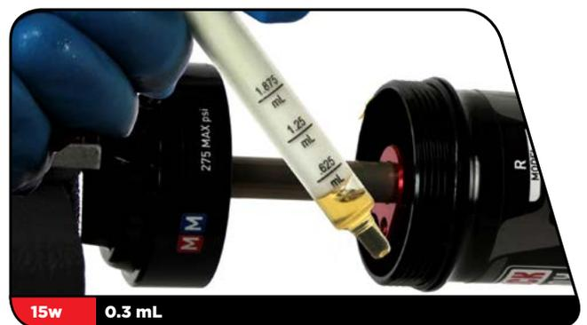
**3** Continue to press the air can onto the damper body until the air can threads and shaft eyelet threads make contact. Turn the air can clockwise and hand-tighten it onto the shaft eyelet.
