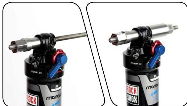
**3** Clamp the catcher in a vise or hold it secure with a 13 mm open end or adjustable wrench.
