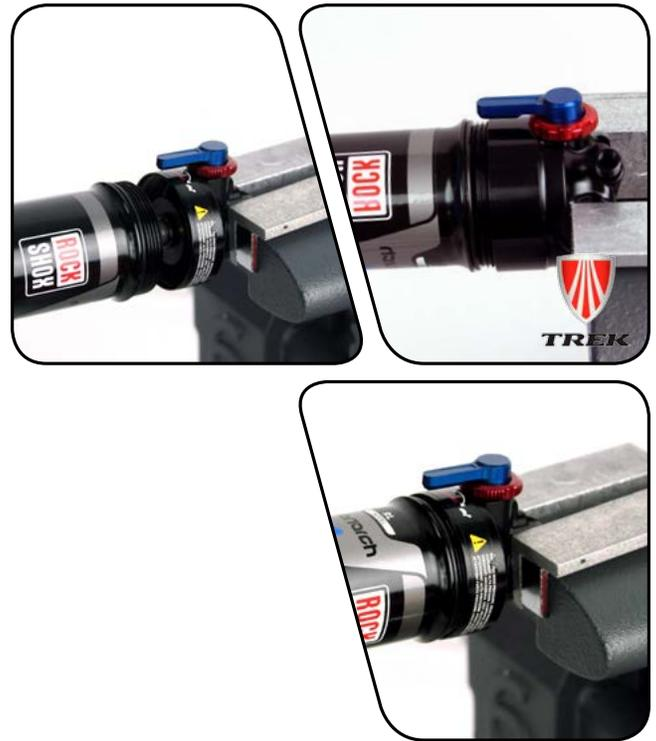
**4** Remove the shock from the vise. Turn it over and clamp the damper eyelet into the vise, so the shock is vertical.
