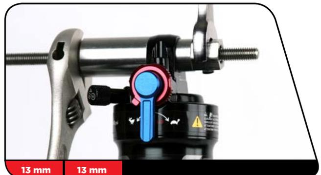
**3** Unthread the catcher from the threaded rod. Remove the tool from the shaft eyelet and discard the old bushing.
