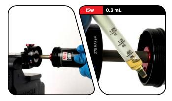
Continue to press the air can onto the damper body until the air can threads and shaft eyelet threads make contact. Turn the air can clockwise and hand-tighten it onto the shaft eyelet.
