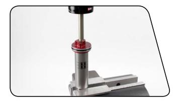
**3** Use a 2 mm hex wrench to remove the bleed screw, located in the seal head/air piston.
