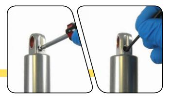
Use a Schrader valve tool to remove and replace the Schrader valve core from the damper air/nitrogen fill port.
