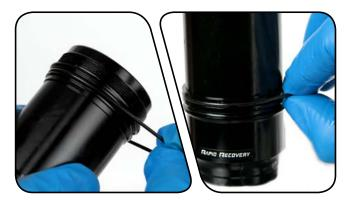
**High Volume Air Cans:** Apply a small amount of suspension specific grease to the inside of the sleeve. This stops the o-rings from rolling as the sleeve slides over them.
