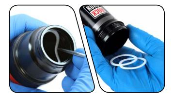
Use a pick to remove the two backup rings from the second deepest groove inside the air can.
