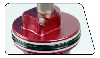
Use a 2 mm hex wrench to thread the bleed screw into the bleed port until you feel it touch the compression ball, then tighten the bleed screw an additional  $\frac{1}{2}$  turn.
