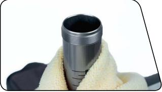
Monarch™ RT3: Pour new RockShox 7wt suspension fluid into the damper body until it is level with the top.
