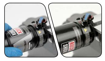
Remove the shock from the vise. Turn it over and clamp the damper eyelet into the vise, so the shock is vertical.
