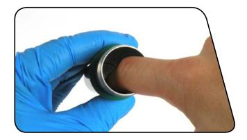
Remove and replace the IFP o-ring. Apply grease to the o-ring.
