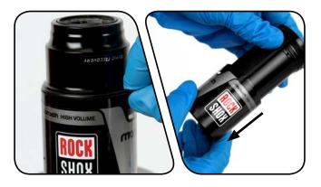
10 High Volume Air Cans: Use your fingers to remove and replace the high volume sleeve o-rings.
