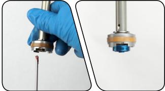
Test the compression rod and top hat function by rotating the compression lever to the closed position and pushing on the top hat. The top hat should have a small amount of movement. If it does not move, adjust the top hat spring so it is seated inside the groove.
