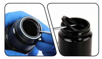
2 Use a pick to remove the two backup rings from the second deepest groove inside the air can.
