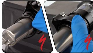
Place a strap wrench on the air can where the AUTOSAG sleeve was located. Turn the strap wrench counter-clockwise to remove the air can.
