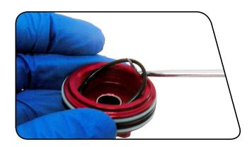
Use a 1.5 mm hex wrench to push the compression ball out of the backside of the seal head through the bleed port.
