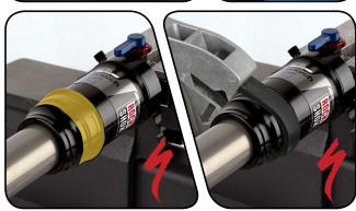
**DebonAir**<sup>TM</sup> **Air Cans:** Remove the sleeve retaining o-ring and the outer sleeve. Clean the air can sleeve. Place a strap wrench on the air can. Turn the strap wrench counter-clockwise to remove the air can.
