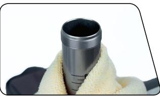
Pour new RockShox 3wt suspension fluid into the damper body until it is level with the top.
