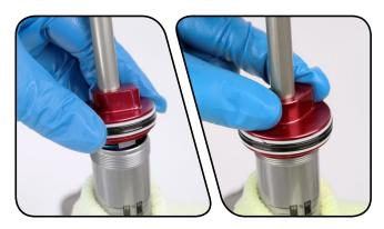
Use a torque wrench with 17 mm crowfoot to tighten the seal head/air piston to 28 N·m (248 in-lb).
