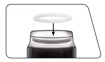
Orient the new dust wiper seal step side up. Install it into the dust wiper seal groove at the top of the air can.
