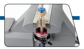
Remove the compression rod and top hat assembly by hand. Keep all the parts together and set them aside.
