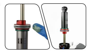
Apply a small amount of grease to the air can threads. Inject 0.5 mL of Maxima® Maxum4 Extra 15w 50 into the air can before installing the air can onto the damper. Firmly press the air can down until the sealhead/air piston is inserted into the air can.
