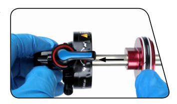
**3** Use the RockShox Rear Shock Vise Block to clamp the shaft into a vise.
