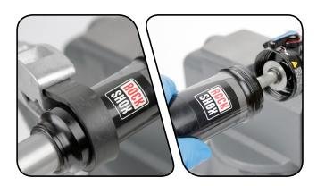
**Specialized® AUTOSAG Air Cans:** Use your fingers or a pick to remove the retention o-ring on the Autosag sleeve. Remove the AUTOSAG sleeve off the air can. Clean the air can with a rag.
