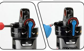
Use a Schrader valve tool to remove the damper air fill port cap. Use a small hex wrench or pick to depress the Schrader valve and release all air pressure from the damper.
