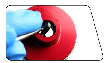
9 Use a pick to remove and replace the inner o-ring, located at the base of the threads in the seal head/air piston.
