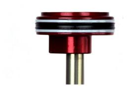
Install the seal head/air piston onto the damper shaft.
