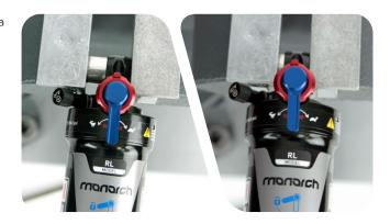
Continue to press the eyelet bushing until it is seated in the shaft eyelet.
