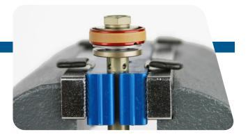
Monarch RT3: Use a 12 mm socket wrench to remove the piston nut.
