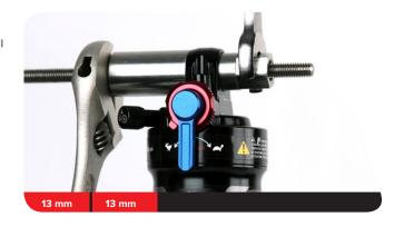
Unthread the catcher from the threaded rod. Remove the tool from the shaft eyelet and discard the old bushing.
