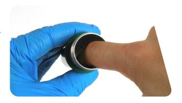
Remove and replace the IFP o-ring. Apply RockShox Dynamic Seal Grease to the o-ring.
