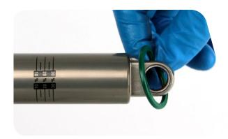
Use a Schrader valve tool to remove the damper air/nitrogen fill port cap. Use a small hex wrench or pick to depress the Schrader valve and release all air pressure from the damper.
