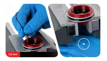
10 Remove and replace the bottom out washer and o-ring from the shaft.
