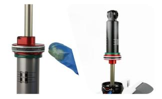
Inject 0.5 mL of Maxima Maxum4 Extra 15w50 or Maxima PLUSH Dynamic Suspension Lube Light into the air can before installing the air can onto the damper. Firmly press the air can down until the sealhead/air piston is inserted into the air can.
