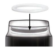
7 Orient the new dust wiper seal step side up. Install it into the dust wiper seal groove at the top of the air can.
