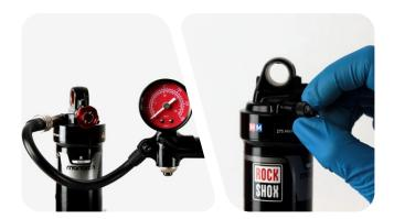
DebonAir Air Can only: Use a shock pump to pressurize the shock to the desired air pressure. After adding air to the shock, the pressure will need to be equalized between the shock chambers.
