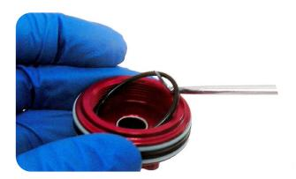
9 Use a 1.5 mm hex wrench to push the compression ball out of the backside of the seal head through the bleed port.
