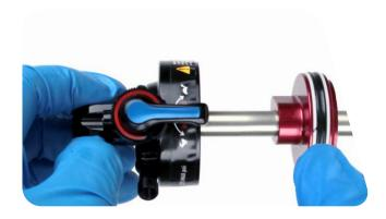
Use a vise block with the 10 mm shaft clamp to clamp the shaft into a
