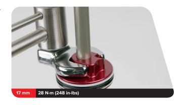
Allow air bubbles to escape from the bleed port in the seal head. Insert the new compression ball into the bleed port.
