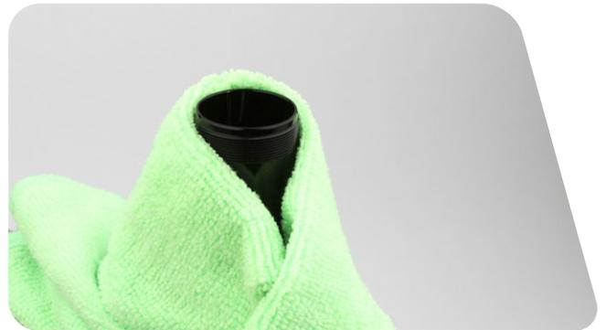
**2** 将新的 RockShox 7wt / Maxima PLUSH 7wt 避震油倒入阻尼器身，直至油液与顶部保持齐平。
