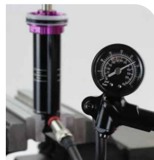
Shock Pump (600 psi max) 400 psi / 27.6 bar
