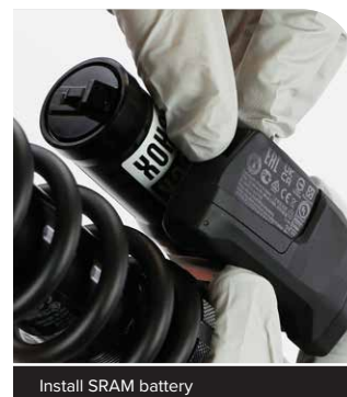
Install SRAM battery
