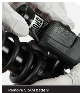
Remove SRAM battery
