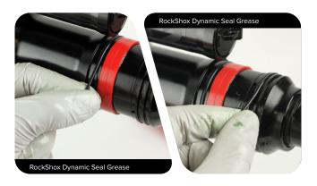
Apply grease to the inner diameter of the outer air sleeve. Install the outer air sleeve onto the air can with the bump on the outer diameter of the outer sleeve oriented away from the eyelet.
