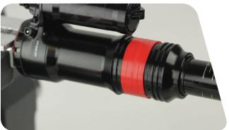
2 Apply grease and install the two small o-rings to the grooves on the air can.
