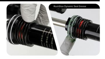
Apply a thin layer of grease to the quad seal, backup ring, and wiper seal.
