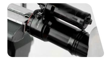
Remove the shock from the vise. Turn it over and clamp the damper body eyelet in the vise.
