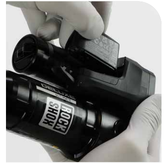
Remove SRAM battery
