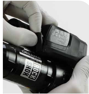
Remove SRAM battery
