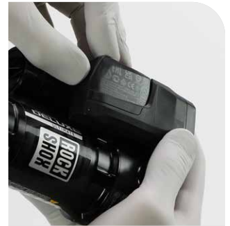
Install SRAM battery
