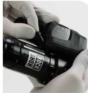
Install SRAM battery
