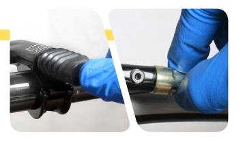
2 Use a T25 TORX\* wrench to loosen the clamp bolt and rotate the remote on the handlebar until the bleed screw is at the highest point.
