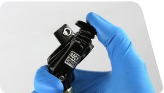
Install the RS-1 Anchor Tool onto the Accelerator Damper™.
