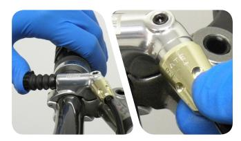
Use a T25 TORX® wrench to loosen the XLoc Sprint handlebar clamp and take the XLoc off of the handlebar.
