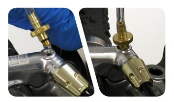
Hold both syringes upright. Pressurize the damper syringe by pushing down on the syringe handle and simultaneously pulling up on the remote syringe handle.
