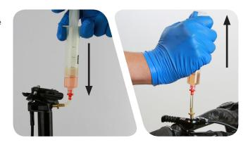
Disconnect the syringe from the seatpost bleed port. Use a T10 TORX wrench to reinstall the bleed screw and tighten to 1.1-2.2 N•m (10-20 in-lb).
