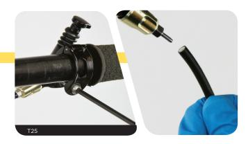
Unthread the hydraulic hose from the banjo fitting on top of the damper, located at the fork crown.
