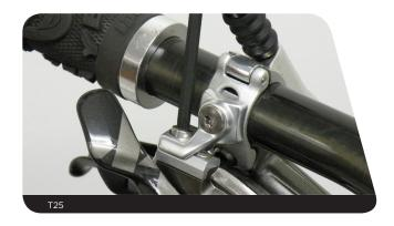
Use a T25 TORX wrench to loosen the XLoc Sprint handlebar clamp, position the XLoc Sprint so that the bleed screw is slightly above the button, and retighten the clamp bolt.
