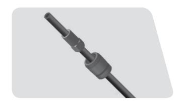
Use a Hydraulic Hose Barb Driver Tool or a T10 TORX\* wrench to thread the new hose barb into the end of the hose until it is flush. Install the compression fitting onto the hose.
