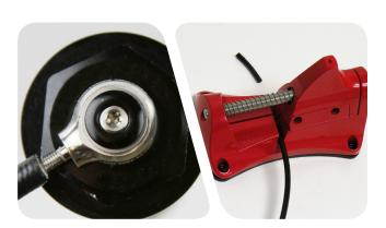
Thread the new hydraulic hose back onto both hose fittings and reinstall the XLoc Sprint onto the handlebar.
