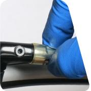
Use a T10 TORX® wrench to thread the remote bleed screw into the bleed port.
