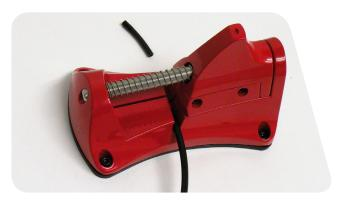
Apply SRAM® Butter grease to the hose barb threads, the new compression fitting outer surfaces, and the compression nut threads.
