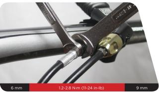
5 Slide the Connectamajig™ boot along the hose and onto the Connectamajig.
