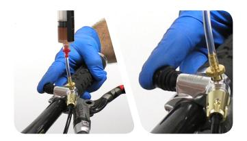
Pressurize the remote syringe by pushing down on the syringe handle, and then press the remote actuator into the extended (locked) position.
