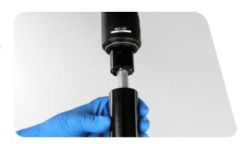
Use your fingers to remove the wire spring from the dust wiper seal and set it aside.
