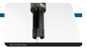
Use a 30 mm socket wrench to push up the rebound shaft, then engage the anchor and rotate the RS-1 Anchor Tool clockwise to unthread the anchor.
