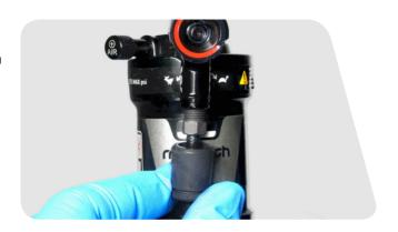
17 While continuing to push the hose into the rear shock banjo fitting, use a torque wrench with an 8 mm crowfoot socket to tighten the compression nut to 5 N·m (44 in-lb).
