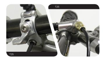
Press the remote actuator into the extended (locked) position. Turn the gold Floodgate adjuster in the direction of the the arrow until it stops (maximum Floodgate).
