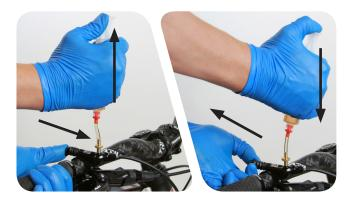
Push down on the remote syringe plunger and make sure the remote actuator is fully extended. Remove the syringe and use a T10 TORX wrench to reinstall the bleed screw and tighten to 1.1-2.2 N•m (10-20 in-lb).
