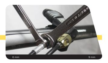
Install a new hose. Inspect and clean the Connectamajig™ hose fitting threads and ball check valve.
