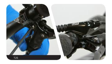
Turn the speed adjuster barrel the opposite direction of the arrow (counter-clockwise) until it stops.
