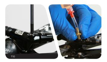
Pull up on the remote syringe plunger and slowly press down on the remote actuator, then press in on the remote syringe plunger until the remote lever fully extends. Repeat this process a few times until no more bubbles are pulled from the system.
