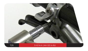
Attach the XLoc shifter to the XLoc bracket with the shifter mounting bolt. Use a T25 TORX wrench to tighten the shifter mounting bolt to 2.8-3.4 N·m (25-30 in-lb).
