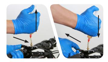
Press down on the remote syringe plunger and make sure the remote actuator is fully extended. Remove the syringe and use a T10 TORX® wrench to reinstall the bleed screw and tighten to 1.1-2.2 N•m (10-20 in-lb).
