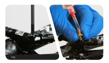
Use a T10 TORX® wrench to remove the bleed screw from the seatpost head, then install the empty syringe into the bleed port.
