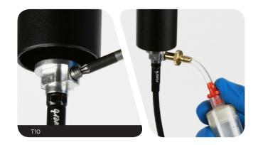
Press down on the remote syringe plunger while pulling up on the seatpost syringe plunger. Press down on the plunger of the syringe attached to the seatpost while pulling up on the remote syringe plunger.
