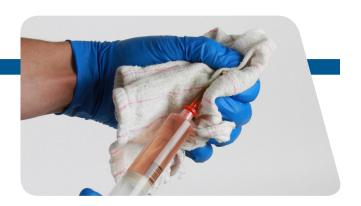
4 Use a T10 TORX wrench to remove the bleed screw from the remote. Install the fluid filled syringe into the bleed port.
