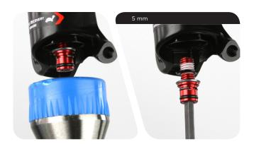
Firmly pull the stanchion downward until fluid begins to drain. Continue pulling downward to remove the stanchion from the Carbon Fiber Upper.
