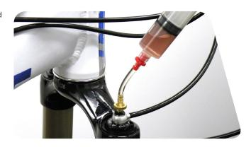
8 Gently push down the syringe plunger to fill the system with Reverb Hydraulic Fluid.
