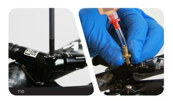
Use a T10 TORX wrench to remove the bleed screw from the bottom of the seatpost, then install the empty syringe into the bleed port.
