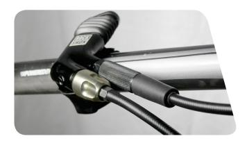
Route the rear hose along or through the frame to the rear shock. Leave a gentle bend from the frame to the handlebar and rear shock.
