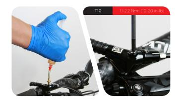
Press the remote actuator five times. Release it to allow the actuator to return to its extended position.
