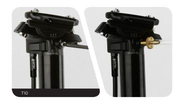
Press down on the remote syringe plunger while pulling up on the seatpost syringe plunger. Press down on the plunger of the syringe attached to the seatpost while pulling up on the remote syringe plunger.
