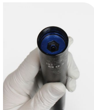
Air shaft unthreaded from seatpost head
