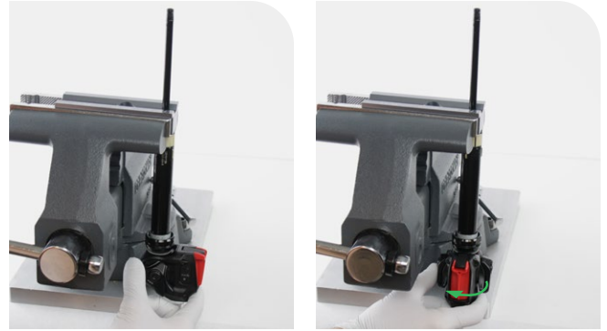
Air piston unthreaded from air shaft
