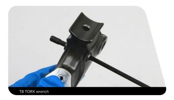
Remove the SwingLink bushings from both sides of the lever. 4
