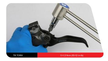
Use a T8 TORX wrench to install a new binder bolt plug. 10
