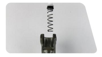
Install the washer on the piston assembly.
