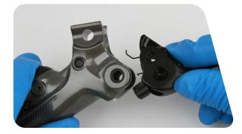
Make sure the lever return spring is seated properly in the lever. The outboard end of the spring must press against the lever blade, while the inboard end of the spring must press against the lever body. If the return spring is not seated properly, you will not be able to adjust the reach of the lever blade. The reach adjuster must be seated in the cam hole, if it is not set properly you will be unable to adjust your reach.
