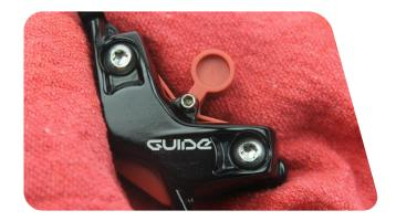
Visually check your work. If any of the o-rings protrude from the banjo fitting or banjo bolt, remove and replace the o-rings, then repeat the installation process.
