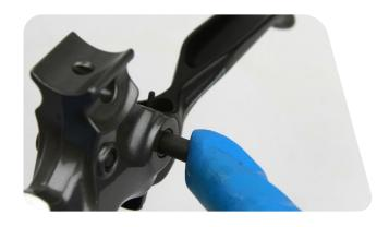
Apply a small amount of Loctite® Threadlocker Blue 242® onto the pinch bolt.
