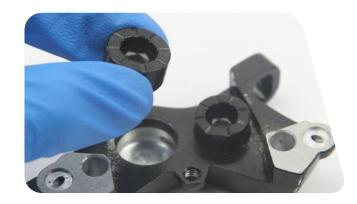
9 Remove the piston seals from each caliper body half. Install new seals inside each caliper body half.
