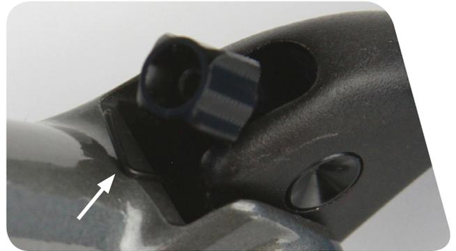
**RS only:** Use your hand to insert the lever assembly into the lever body, placing the push rod into the piston and lever return spring on the lever body.
