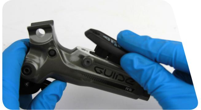
**12** Use a torque wrench with a T10 TORX® bit to tighten each reservoir cap bolt to 2.7-3.2 N·m (24-28 in-lb).
