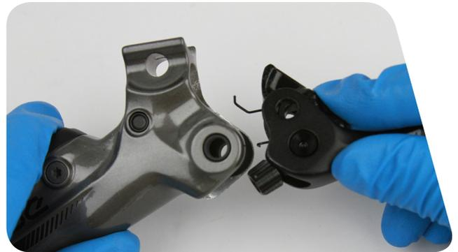
*Make sure your lever return spring is seated in the lever properly, as seen in the picture. The end of the spring that points outward must be placed against the lever blade, while the end of the spring that points inward rests against the lever body. The reach adjuster must be seated in the cam hole, if it is not set properly you will be unable to adjust your reach.*
