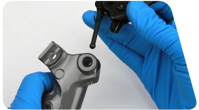
*Make sure your lever return spring is seated in the lever properly, as seen in the picture. The reach adjuster must be seated in the cam hole, if it is not set properly you will be unable to adjust your reach.*
