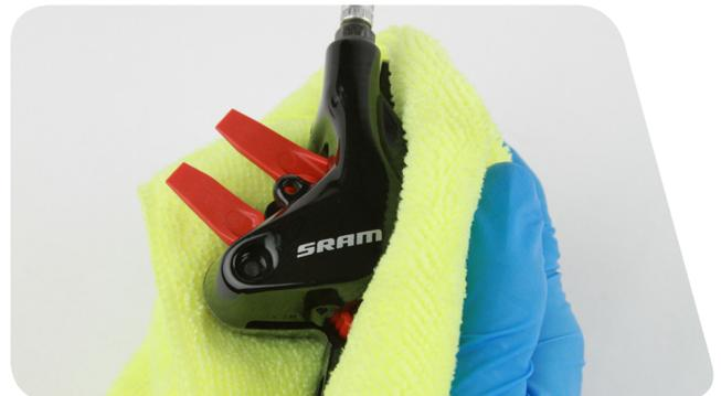
Visually check your work. If an o-ring protrudes from the crimped hose fitting, remove and replace the o-ring, then repeat the installation process.
