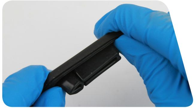
**11** Insert the reservoir cap/bladder assembly onto the lever body.
