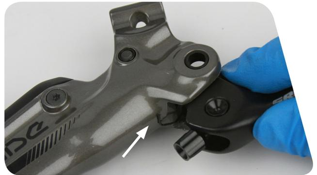
**7** Line up the cam and lever blade with the holes in the lever body, then press the pivot pin through the holes.
