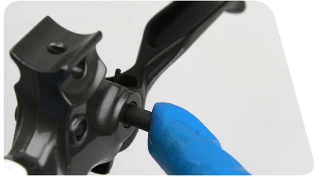
**8** Apply a small amount of blue Loctite onto the pinch bolt. Use a T8 TORX® wrench to thread the pinch bolt into the lever body. Use a torque wrench and a T8 TORX® wrench to tighten the bolt to 2.7-3.2 N·m (24-28 in-lb).
