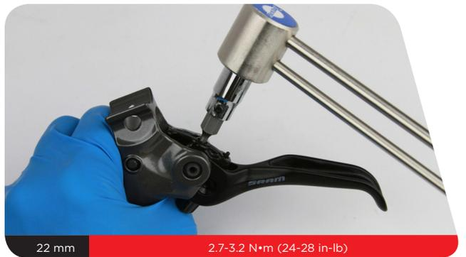
**9** Use a T8 TORX® wrench to install a new binder bolt plug.
