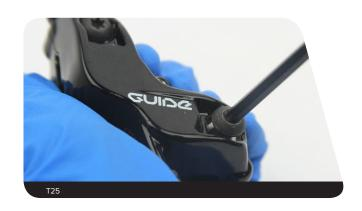
Separate the caliper body halves.
