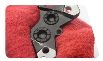
Add a small amount of DOT compatible grease onto the new caliper square body seals, then install onto the caliper.
