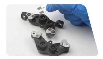
Remove the caliper square body seals from the outboard side of the caliper.
