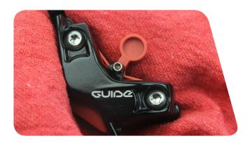
Visually check your work. If any of the o-rings protrude from the banjo fitting or banjo bolt, remove and replace the o-rings, then repeat the installation process.
