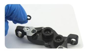
Remove the pistons from each caliper body half.
