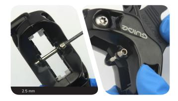
2 Squeeze the brake lever numerous times to advance the pistons until they contact the pad spacer.
