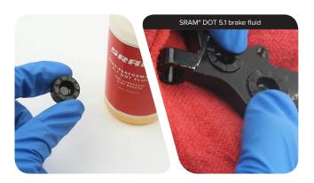
2 Spray isopropyl alcohol on the caliper halves and both of your gloves and clean them with a rag.
