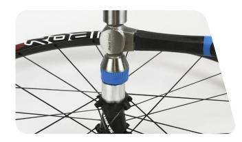
Strike the FR/440 Front Hub Tool with a soft face mallet until the bearing is firmly seated into the bearing pocket.
