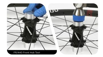
Remove the upper LFR/440 Front Hub Tool from the axle. Install a new bearing onto the axle with the red seal facing away from the hub.
