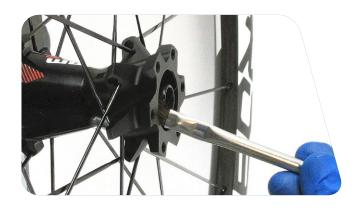
31 Apply a very thin layer of **DT Special Grease** to the teeth of the ring nut.
