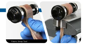
**5** Remove the end cap. If the axle rotates in the strap tool, remove it from the vise and pull the strap tighter. Make sure the bearing does not come off of the axle.
