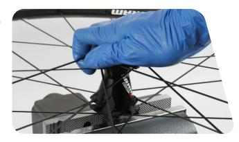
Press down firmly and rotate the wheel counter-clockwise to remove the ring nut from the hub. The rotor seal will also be removed, and may fall over the ring nut tool onto the vise. Remove the ring nut from the tool. Clean the ring nut and inspect for any damage. Replace the ring nut if it is damaged.
