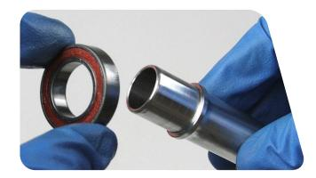
Remove the bearing from the axle and discard.
