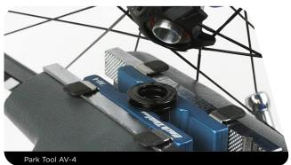
Pull the driver body and spring from the hub by hand. Remove the two star ratchets.
