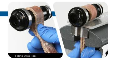
Remove the end cap. If the axle rotates in the strap tool, remove it from the vise and pull the strap tighter.
