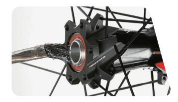
20 Thread the new end caps onto the axle. Tighten the end caps to 15 N•m (133 in-lb).
