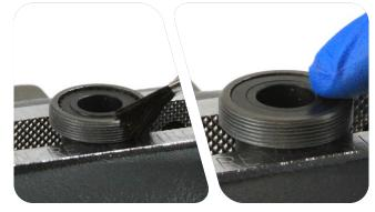
To install the ring nut, first install the Ring Nut Installation Tool into a vise so that the teeth are level with the top of the vise.
