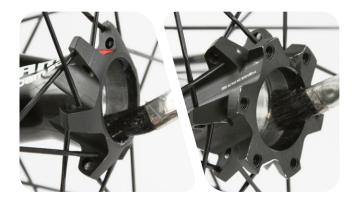
Install a new bearing onto the long end of the axle with the red seal facing away from the axle.
