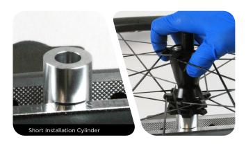
Place the rotor seal onto the Seal Installation Tool with the rubber seal facing the tool. Place the tool onto the axle with the rotor seal facing toward the hub.
