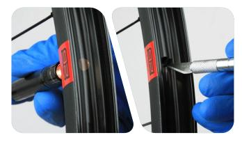
Remove the nut and o-ring from the valve stem. Install the valve stem into rim.
