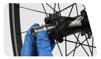
6 Install the Long Stepped Tool into the axle. Strike the axle with a soft face mallet to remove the bearing from the hub.
