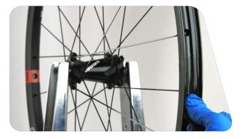
Apply tension to the tape by rotating the wheel away from you while rapidly "shaking" the tape from side to side about 2-3 inches (5-8 cm). This will seat the tape into the channel and keep it centered in the rim.
