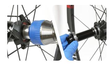
Insert the Small Stepped Tool into the open end of the axle.
