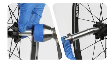
Use a soft face mallet to tap out the axle from the hub.
