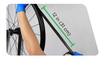
Cut the tape. Use your fingers or a tire lever to press the leading edge of tape against the rim. This will help prevent sealant from getting under the tape.
