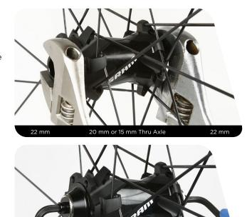
Insert the Small Stepped Tool into the open end of the axle.
