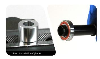
Install the long end of the axle into the Short Installation Cylinder. Firmly press down on the axle to seat the bearing onto the axle.
