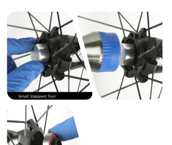
Remove the bearing from the axle and discard. Install a new bearing onto the axle with the red seal facing away from the axle.
