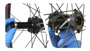
Insert one of the FR/440 Front Hub Tools into the hub against the face of the installed bearing.
