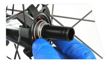
Install the spring onto the axle and over the spacer. The wide opening of the spring is toward the hub.
