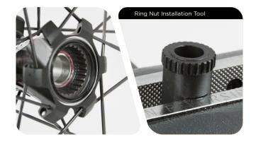
Install the drive side of the hub onto the Ring Nut Installation Tool. Press down firmly and rotate the wheel to make sure that the teeth of the tool engage with the ring nut.
