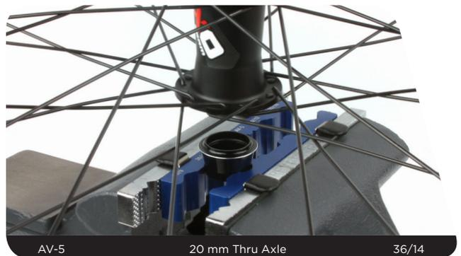
**2** Press the new end caps onto the hub by hand.
