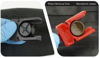
Insert the piston plug so that it fits snugly into the empty piston bore and is flush with the inside of the caliper.
