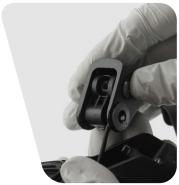
Insert a 2.5 mm hex wrench through the hole in the cross dowel and into the reach adjust pull rod. Rotate the bolt counter-clockwise to tighten the bolt to hand tight.
