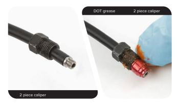
**2** piece caliper: Install the hose into the caliper while threading the compression nut into the caliper by hand. Tighten the compression nut. Install the hose boot over the compression nut.
