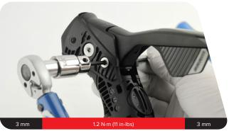
Install the hood cover. Adjust the reach of the lever to your desired setting.
