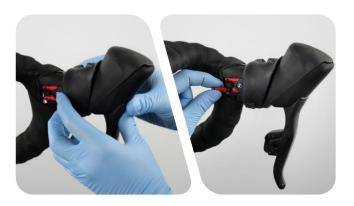
Remove the screw from the auxiliary connector cover, then fold the hood cover backward.
