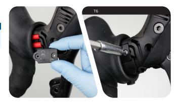
Install the shorter screws into the battery box and gently tighten.
