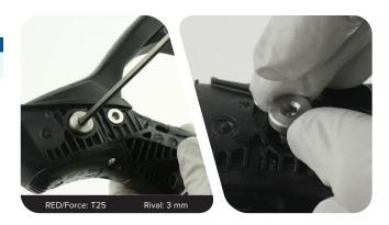
Remove the Stealth-a-majig hose hood assembly from the inboard side of the hood.
