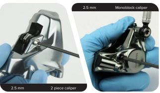
Remove the brake pads from the caliper.
