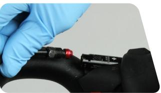
2 piece caliper: Remove the compression nut and hose.
