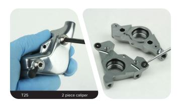
Remove the piston seals from each piston bore.
