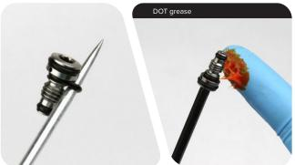
**Monoblock caliper:** Tighten the banjo bolt with the banjo boot at the desired angle.
