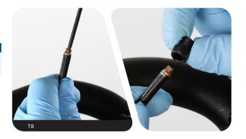
Thread a new compression fitting over the hose barb, counterclockwise, until it is flush or slightly lower than the hose barb.
