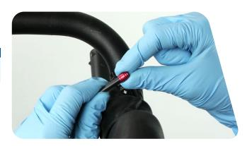
Apply a thin layer of grease to the compression fitting and compression nut.
