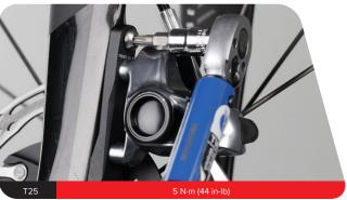
Spin the wheel and check the brake function. The pistons should move freely and there should not be excessive brake lever throw.
