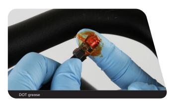
Install the hose into the lever body while threading the compression nut into the valve body by hand. Tighten the compression nut.
