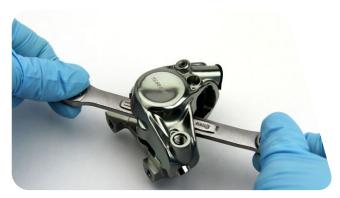
**2 piece caliper:** Install new body seals into the caliper body. Install the cross-body bolts into the caliper body, then tighten.
