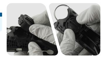
Install the cross dowel into the cross dowel bushing in the lever. Hold in place while the lever is installed.
