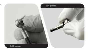
Install the Stealth-a-majig hose banjo into the groove in the inboard side of the hood. Install the banjo bolt into the outboard side of the hood and tighten.
