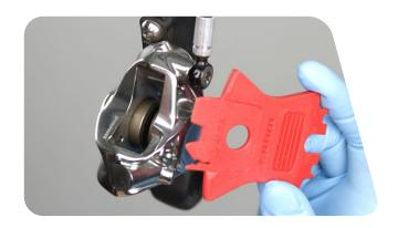
Use a plastic tire lever to push the pistons back into the caliper bores.
