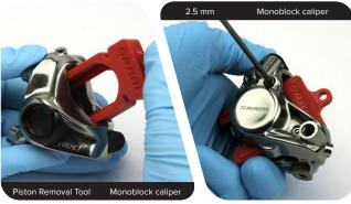
Firmly press a rubber-tipped air chuck nozzle into the banjo port. Hold the caliper securely against a rubber surface and force air into the banjo port to dislodge the piston from the caliper.
