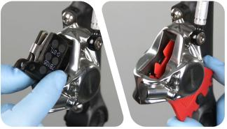
Squeeze the brake lever several times until both pistons have advanced and contact the pad spreader. One piston may move faster than the other; continue to squeeze the lever until the second piston touches the spacer.
