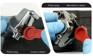
**2 piece caliper:** Remove the cross-body bolts from the caliper. Remove the body seals from the caliper body.
