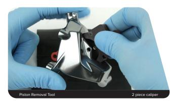
**Monoblock caliper:** Install the pad retention bolt to hold the piston removal tool in place.
