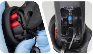
Install the longer screw into the auxiliary connector cover and gently tighten.
