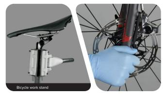
Remove the brake pads and install the pad spacer.
