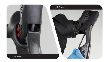
Install the pivot pin nut and the pivot pin bolt into the hood. Hold the nut in place, then tighten the pivot pin bolt.
