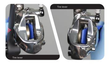
Reinstall the brake pads and install the wheel according to the manufacturer's instructions.
