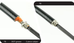
2 piece caliper: Install the compression nut onto the hose.
