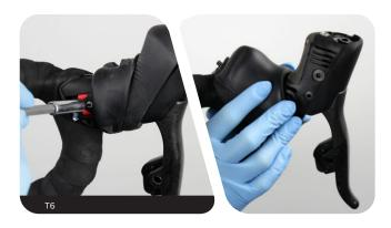
Hold the pivot pin nut in place, then unthread the pivot pin bolt from the hood assembly.
