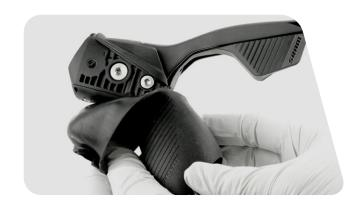
Install the hose into the lever body while threading the compression nut into the valve body by hand. Tighten the compression nut.
