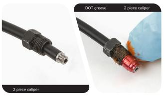
**2 piece caliper:** Install the hose into the caliper while threading the compression nut into the caliper by hand. Tighten the compression nut.
