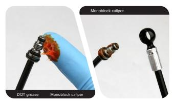
Monoblock caliper: Tighten the banjo bolt with the banjo boot at the desired angle.
