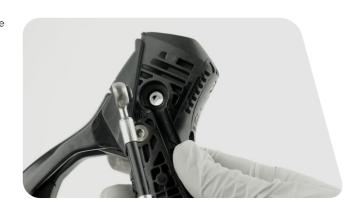
Install a new o-ring on the new Stealth-a-majig hose banjo. Install a new o-ring on the new banjo bolt.
