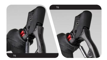
Remove the lever and the battery box from the hood assembly, then remove the auxiliary connectors from the hood assembly.
