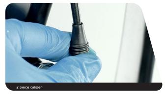
Apply DOT grease to the hose barb threads. Thread the hose barb into the hose until it is flush with the end of the hose.
