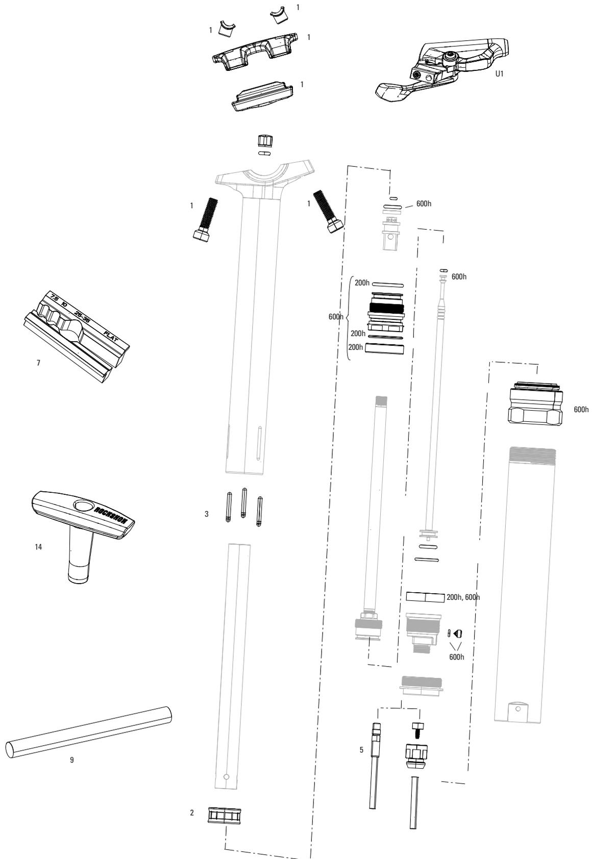
1. Discard bar, o-ring and sleeve when using 11.6815.025.030 seatpost hydraulic hose for Reverb Stealth C1 post
