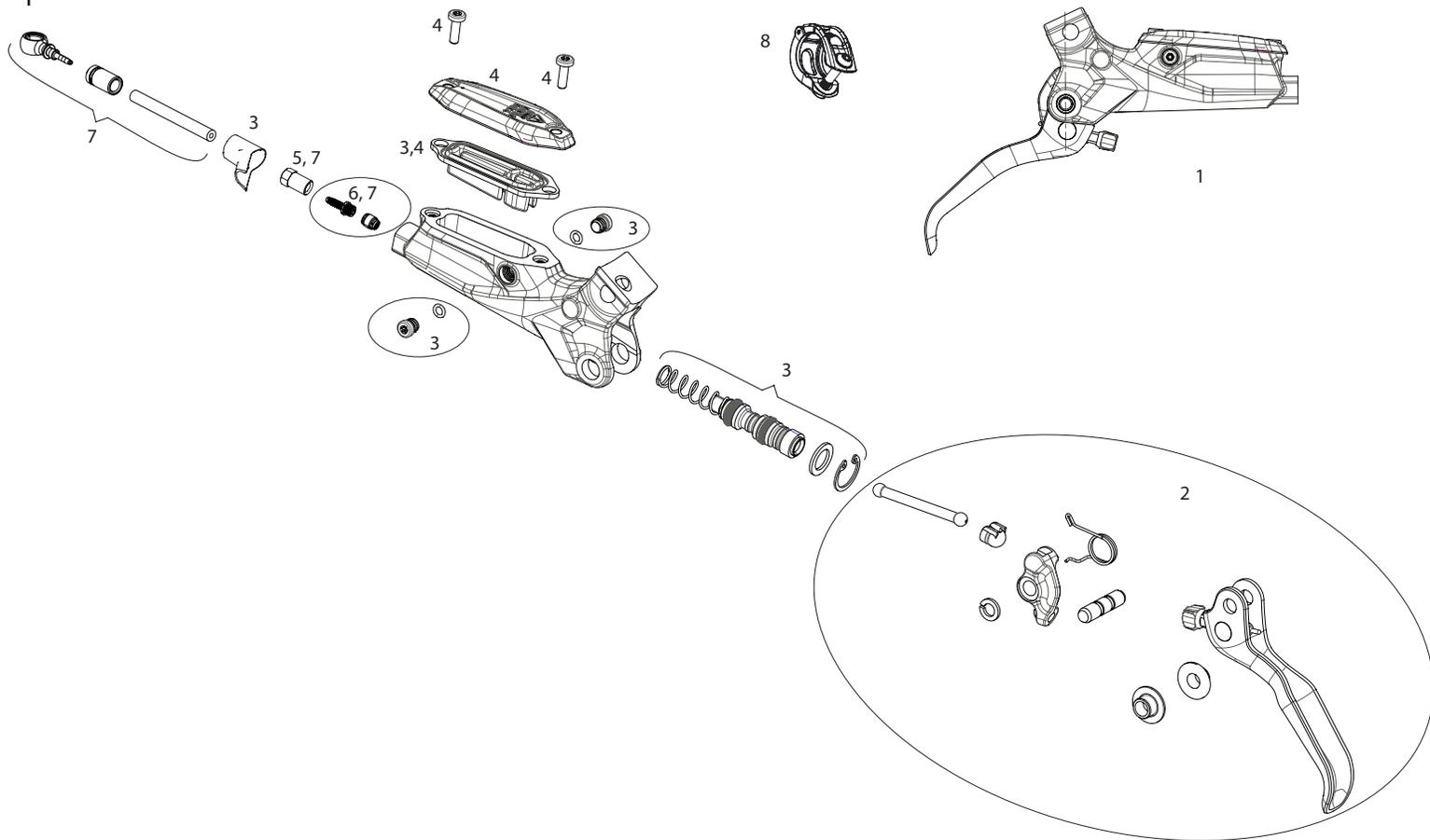
In OEM piston assembly is Stealth-a-majig ; piston assembly AM is non-stealth-a-majig and compatible.
