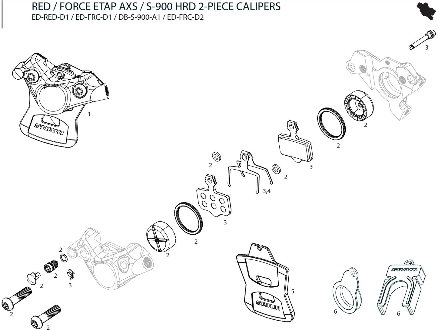
Note: In July 2019 Red AXS disc brakes move to 2-Piece calipers which requires a different line kit & brake pads. See page 166 for mounting bolts.
