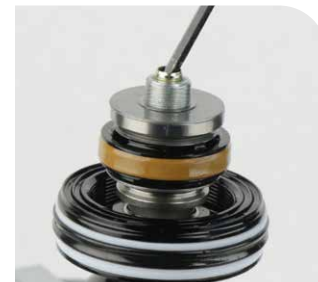
Piston assembly installed
