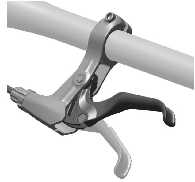
**6** To center the caliper, pull the lever five times, then hold.
