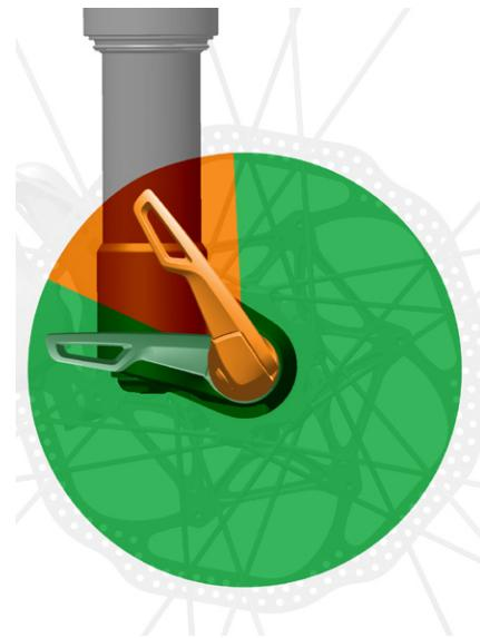
Remove the axle from the dropout. To change the closed position of the Maxle Ultimate lever, open the lever, press down, and rotate the lever head to the desired position.
