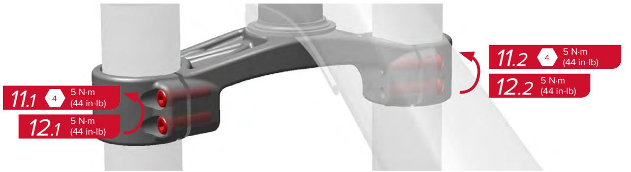
Tighten the 4 lower crown bolts to 5 N·m (44 in-lb), then re-tighten the 2 uppermost bolts to 5 N·m (44 in-lb).
