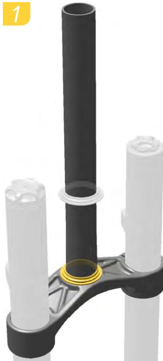
Install a headset into the bicycle frame and a 29.9 mm crown race onto the fork according to your headset manufacturer's instructions.
