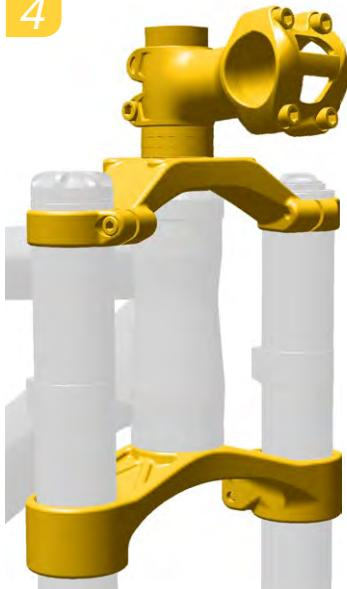
Install the fork into the frame, and install the upper crown onto the steerer tube and upper tubes. Install the stem and any desired spacers. Do not tighten any of the crown or stem bolts.
