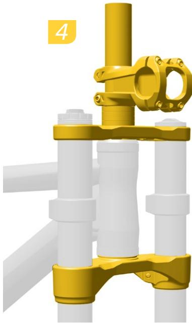
Install the fork into the frame, and install the upper crown onto the steerer tube and upper tubes. Do not tighten any of the crown bolts.
