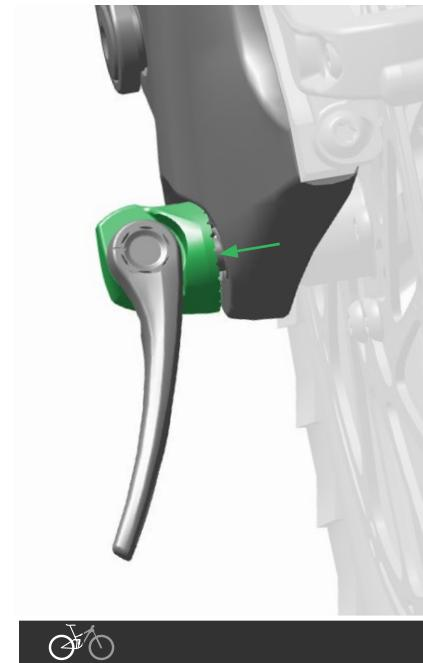
To thread the Maxle into the drop out, rotate the lever clockwise until there is a small gap between the lever head and drop out.
