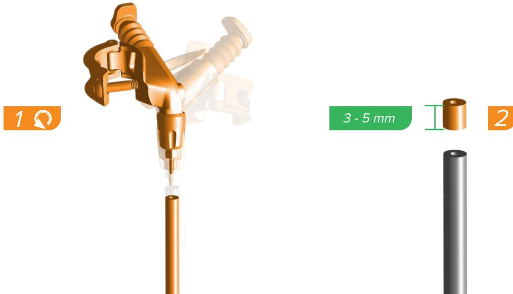
Remove the original remote from the hose and cut 3-5 mm from the end. Cut additional length as needed.
