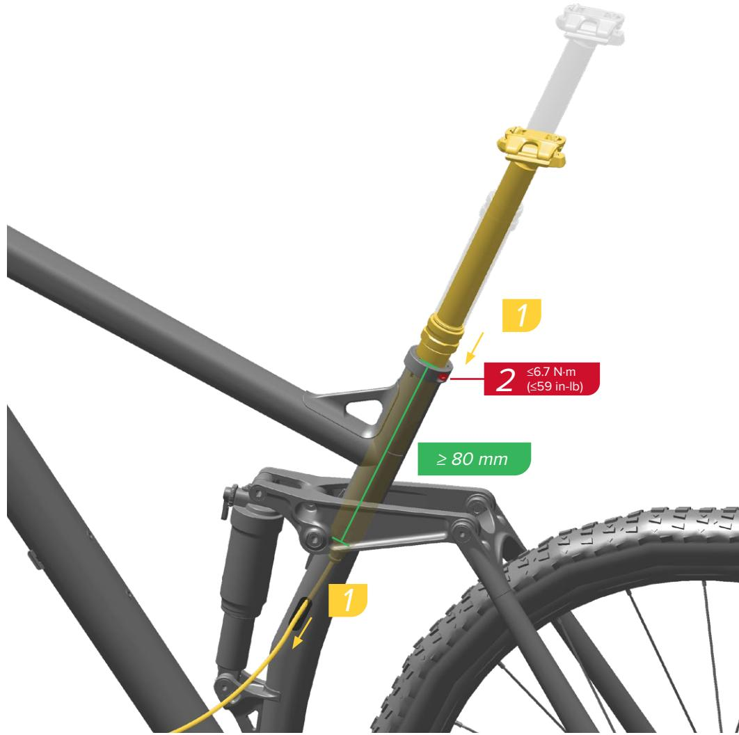
Insert the seatpost into the frame a minimum of 80 mm, or the minimum specified by your frame manufacturer, whichever is greater, and simultaneously pull the remote hose through the frame.
