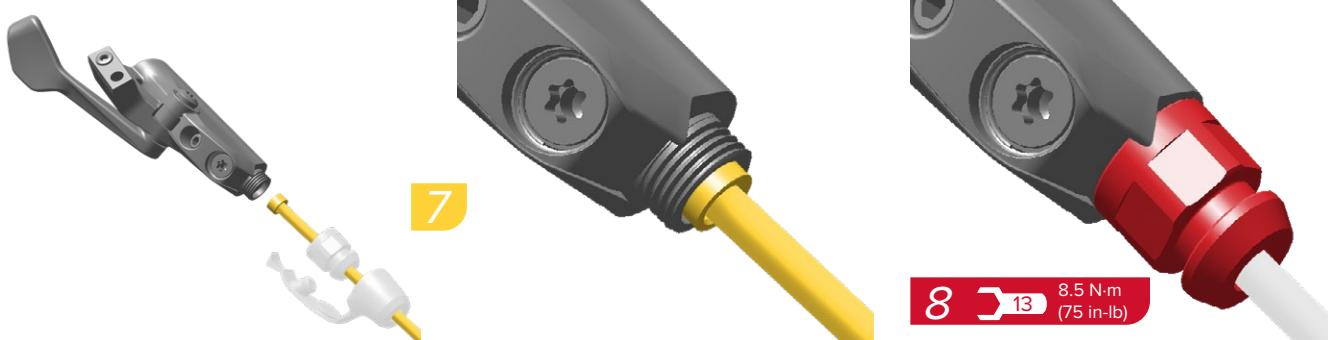
**1x Remote:** Insert the hose barb into the remote. Press and hold the barb in place. Thread the hose nut onto the remote and tighten the nut to the specified torque.
