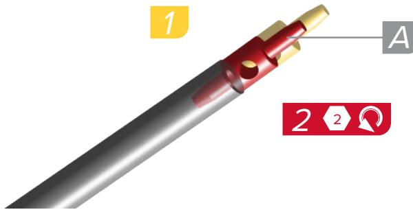
Thread the Reverb Stealth remote hose Barb Connector tool (A) into a 500-700 mm section of shift cable housing, with non-metallic liner, reverse threaded end first. Insert a 2 mm hex wrench through the hole in the tool to rotate it.
