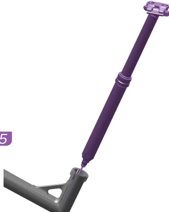
Pull the housing and remote hose through the seat tube and out the frame hose port. Stop when the seatpost is just above the seat tube.
