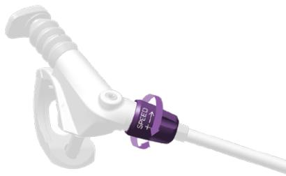
Turn the Speed adjuster counter-clockwise to decrease, and clockwise to increase, the seatpost compression and return speed.
