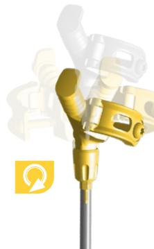
**Remote:** Thread the remote lever hose barb into the hydraulic hose. Stop when the remote hose barb flange contacts, and is tight against, the end of the hose.
