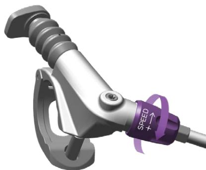
**Remote:** Test seatpost function in the slowest speed setting. Turn the Speed adjuster in the opposite direction of the arrow until it stops. Adjust as desired after function test.
