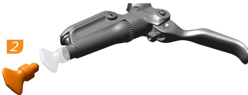
Remove the rubber lever body plug from the lever by pulling the plug straight from the lever. **Do not rotate the rubber lever body plug while removing.**
