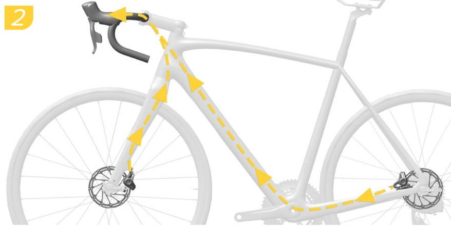
Route the internal routing kit through the desired frame path. Pull the internal routing kit through the bicycle frame while guiding the hydraulic hose from the trailing side.
