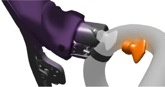
Remove the rubber lever body plug from the valve body by pulling the plug straight from the lever. **Do not rotate the rubber lever body plug while removing.**
